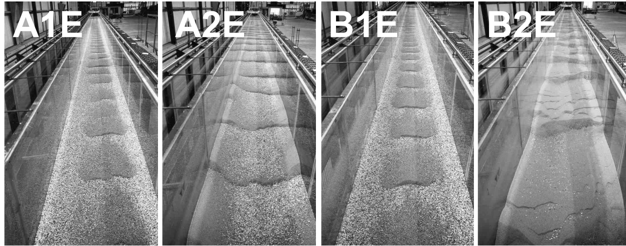
Figure 4.7: Bedform patterns in equilibrium stages of experiments with tri-modal mixture (coarsest fraction is white-coloured).
