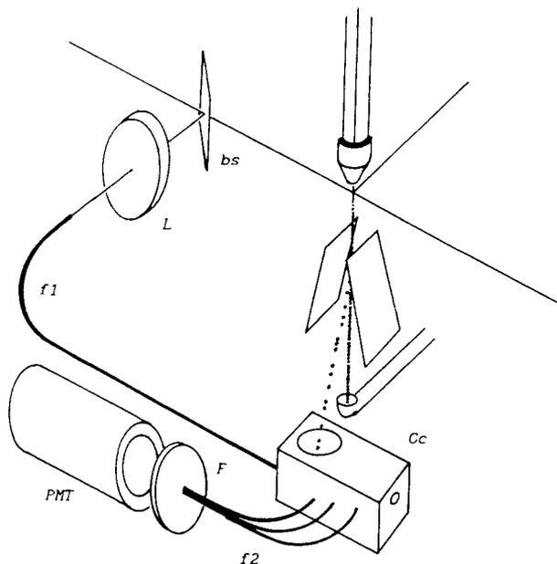
FIG. 2. Schematic drawing of the setup used to measure the time delay. A conventional sorter was used for analyses and sorting equipped with the following extras: bs, beam splitter (microscope slide); L, lens (focal length 40 mm); f1 and f2, optical fibers (inner core 600  $\mu\text{m}$ ); Cc, collection chamber; F, fluorescence filter; PMT, photomultiplier.
