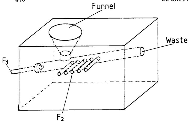
FIG. 1. Drawing of the collection chamber used for fluorescence measurements of the recently sorted droplets. The excitation light is coupled into the capillary via the optical fiber F1. The emitted fluorescence is collected with the fibers F2 mounted orthogonally towards the capillary part of the chamber. The chamber is made of stainless steel.
