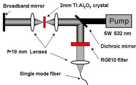
Figure 1. Experimental schematic of low coherence light source. A high doping density Ti:Al<sub>2</sub>O<sub>3</sub> crystal enables pumping with a high excitation density per unit volume. A double pass pump and fluorescence collection geometry is used.
