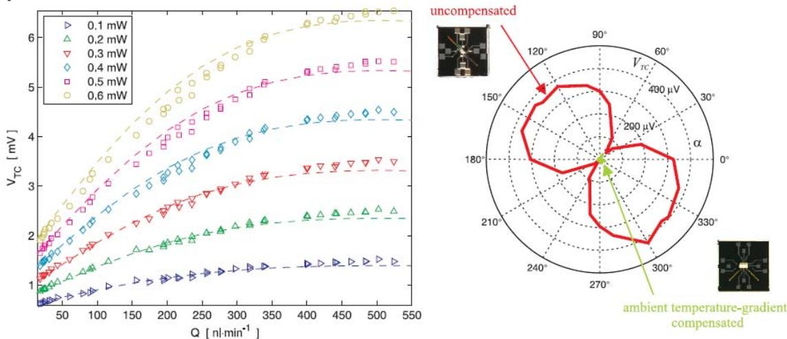
Fig. 3. Left: Flow sensor thermopile-voltage  $V_{TC}$  dependency on water flow rate  $Q$  at various applied total heating powers. Dashed lines show fitted FEM results. Right: External temperature-gradient sensitivity of the thermopile voltage  $V_{TC}$  measured for a compensated sensor and a single-microchannel uncompensated flow sensor.
