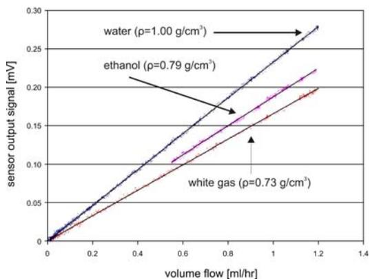
Fig. 4. Left: SEM photograph of a realized Coriolis flow sensor. Right: Measurement results for three different fluids: water, ethanol and white gas, demonstrating that the sensor indeed measures real mass flow (the output signal is proportional to the volume flow times the density of the fluid; independent of the fluid).
