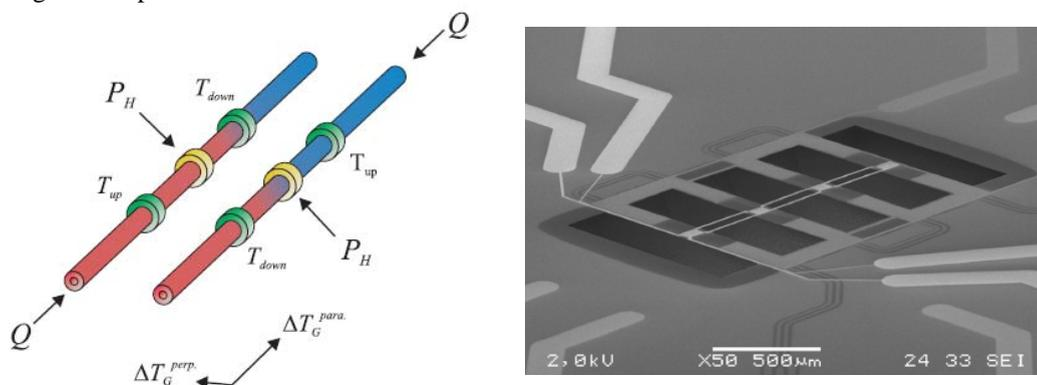
Fig. 2. Thermal flow sensor compensated for gradients in ambient temperature. Left: Principle of operation with fluid flow  $Q$ , and heating elements  $P_H$ . Fluid flow generates a temperature difference between the up- and down-stream sensors whereas an additional gradient due to ambient is cancelled. Right: Photograph of a realized sensor with four parallel channels and integrated Al heater resistors and Al/poly Si++ thermopiles.
