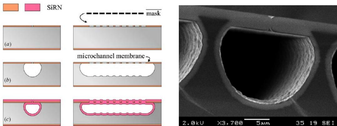
Fig. 1. Surface microchannel process scheme, applying a single mask defining etch holes in a 500 nm SiRN layer and a SEM photograph of the resulting micro channels.
