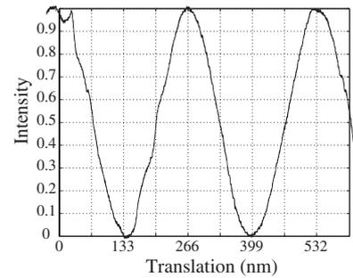
Fig. 4. Intensity of the center of the fringe pattern after angular alignment, as a function of lateral displacement.
