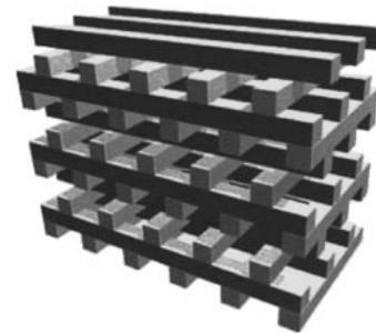
Fig. 1. Example of a 3D PhC structure: the woodpile structure.
