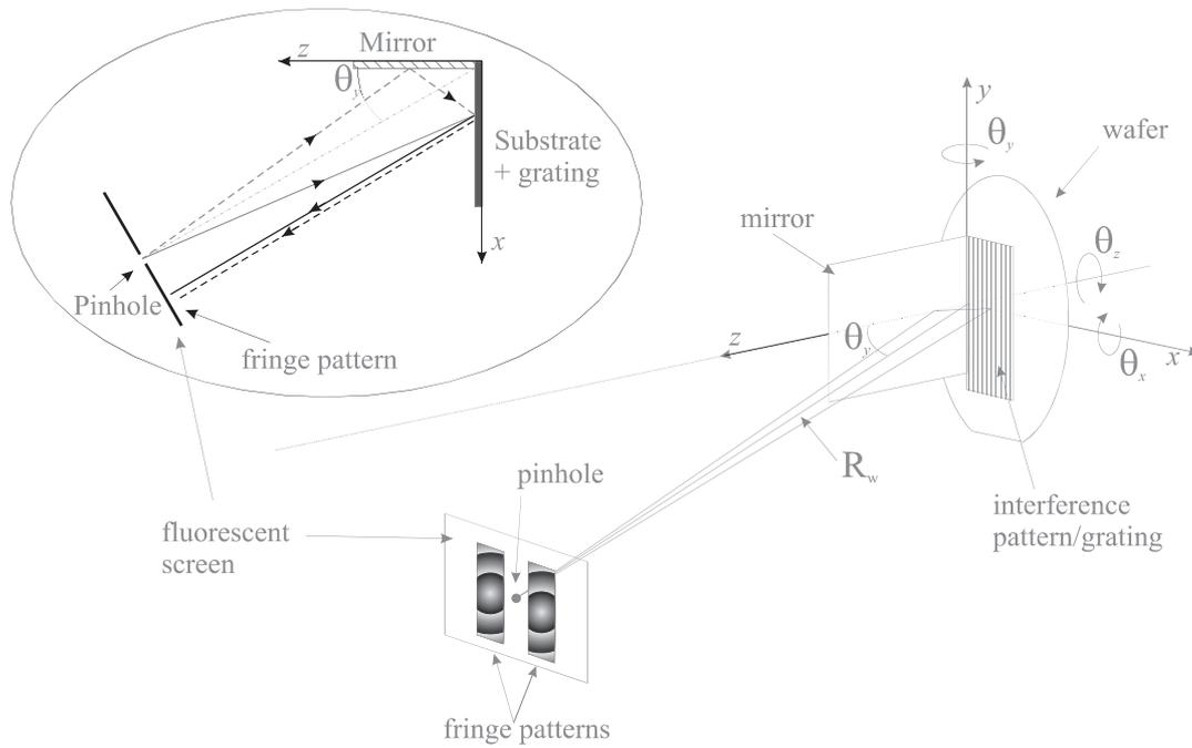
Fig. 2. Set-up for LIL-alignment of a new interference pattern with respect to an existing pattern.
