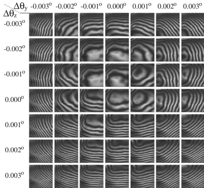
Fig. 3. Different fringe patterns for several combinations of misalignment angles  $\Delta\theta_y$  and  $\Delta\theta_z$  as observed when a wafer with an existing grating is repositioned in the set-up of Fig. 2.
