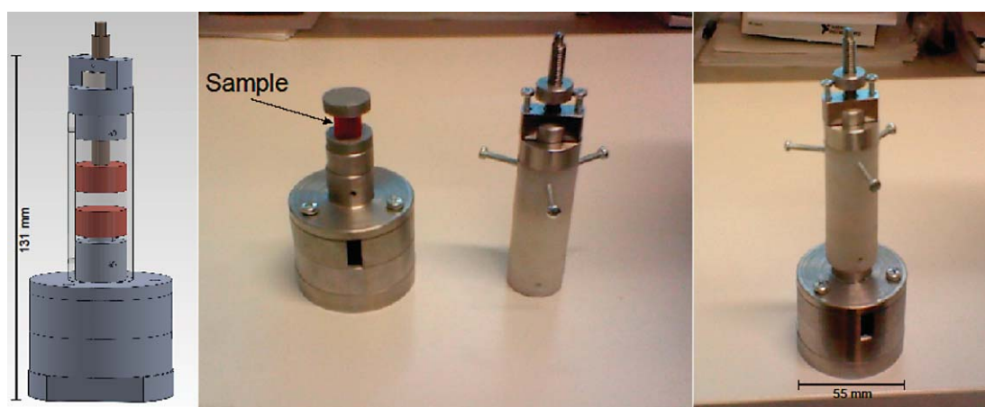
Fig. 1. Mechanical deformation device and the sample setup within it. Drawing in the left pane shows the CAD assembly of the various components. The photographs show the fabricated device where – centre pane: location of a sample within the device, right pane: The assembled device ready to be placed in the \mu\text{CT} .
