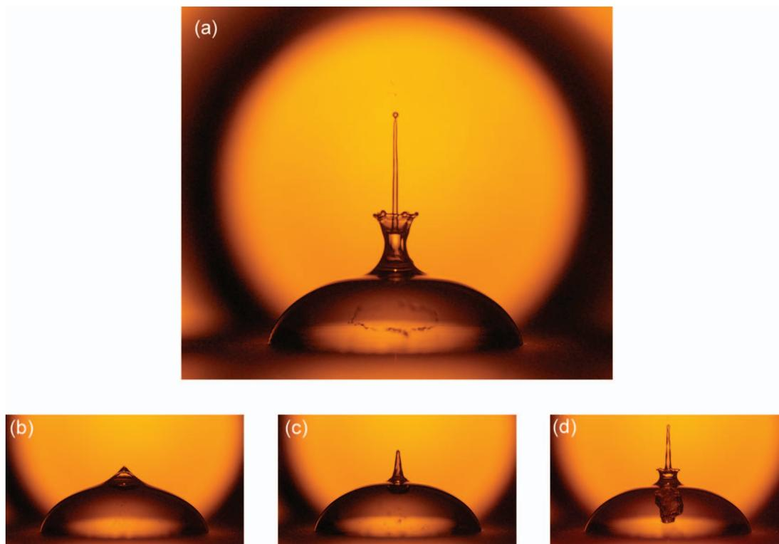
FIG. 1. (Color) Liquid jetting caused by an expanding and collapsing cavitation bubble created close to the apex of the drop. The lower frames [(b)–(d)] show snapshots of the droplet and the bubble activity at times  $40\ \mu\text{s}$ ,  $120\ \mu\text{s}$ , and  $200\ \mu\text{s}$  after bubble creation. Please note that the stretched and toroidal bubble in (d) and its remains are still visible  $200\ \mu\text{s}$  later in the top frame. The width of the droplet base is 6 mm.
