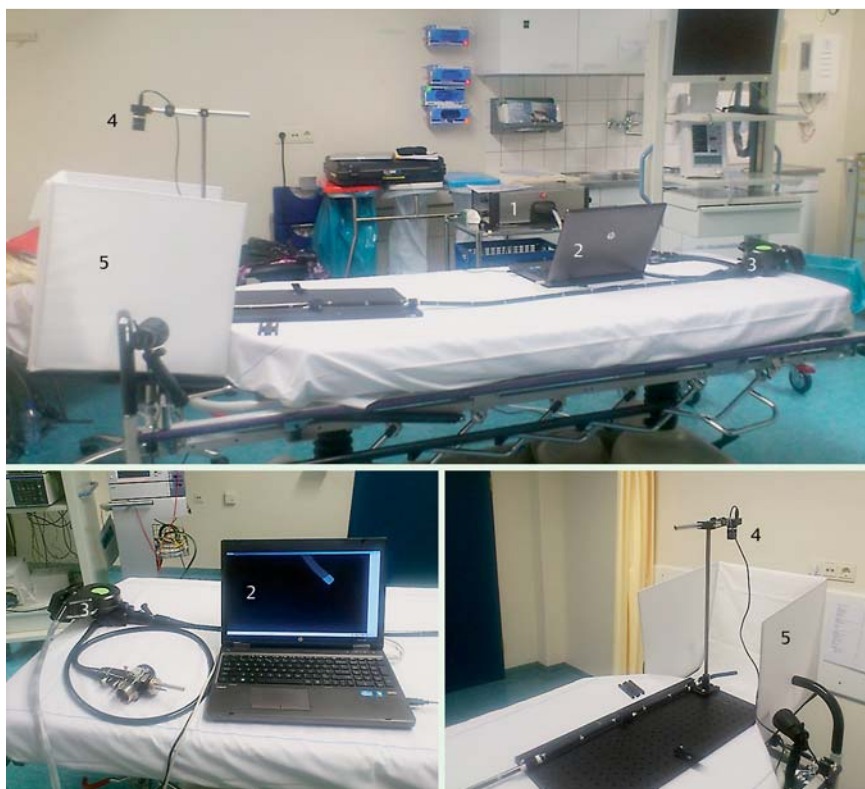
Fig. 2 In-hospital example of setup for hysteresis measurement: 1, motor module; 2, computer; 3, remote drive unit connected to the navigation wheels of a conventional endoscope; 4, camera capturing images of the endoscope tip; 5, light studio to prevent shadow formation from the hovering tip.
