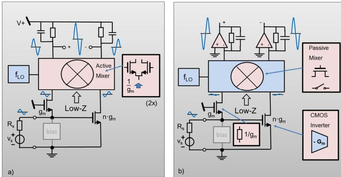
Figure 5: Frequency Translational Noise Cancellation concept: at RF only V-I conversion occurs followed by current-mixing, while I-V conversion is combined with low-pass baseband channel filtering [10]. (b) Interference robust implementation exploiting highly linear passive mixers and OPAMP-RC amplifiers [11].
