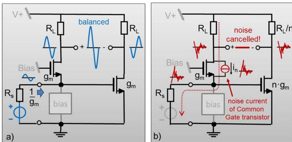
Figure 3: Noise Cancelling Topology with parallel Common Gate and Common Source amplifiers: (a) signals (in blue) are amplified to a balanced differential output; (b) Noise (in red) of the impedance matching Common-Gate transistor produces two correlated noise contributions that cancel at the differential output.
