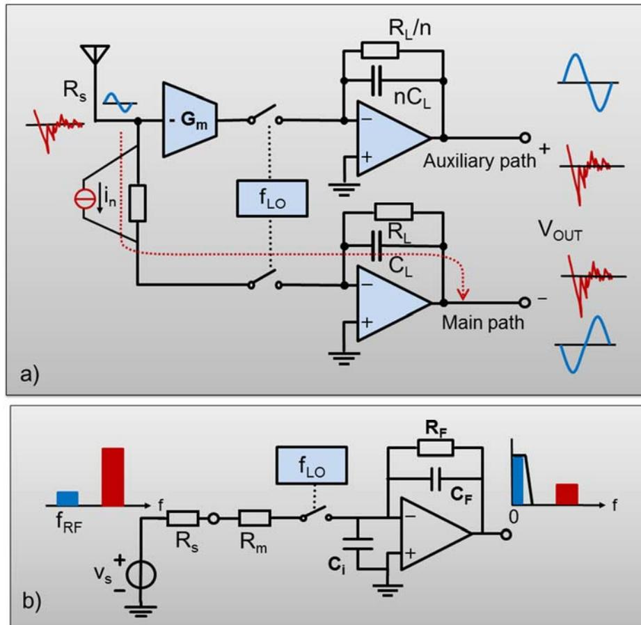
Figure 6: Interference Robust Frequency Translational Noise Cancellation receiver: a) Complete Circuit with main and auxiliary noise cancelling path; b) Signal spectrum along the main receiver chain
