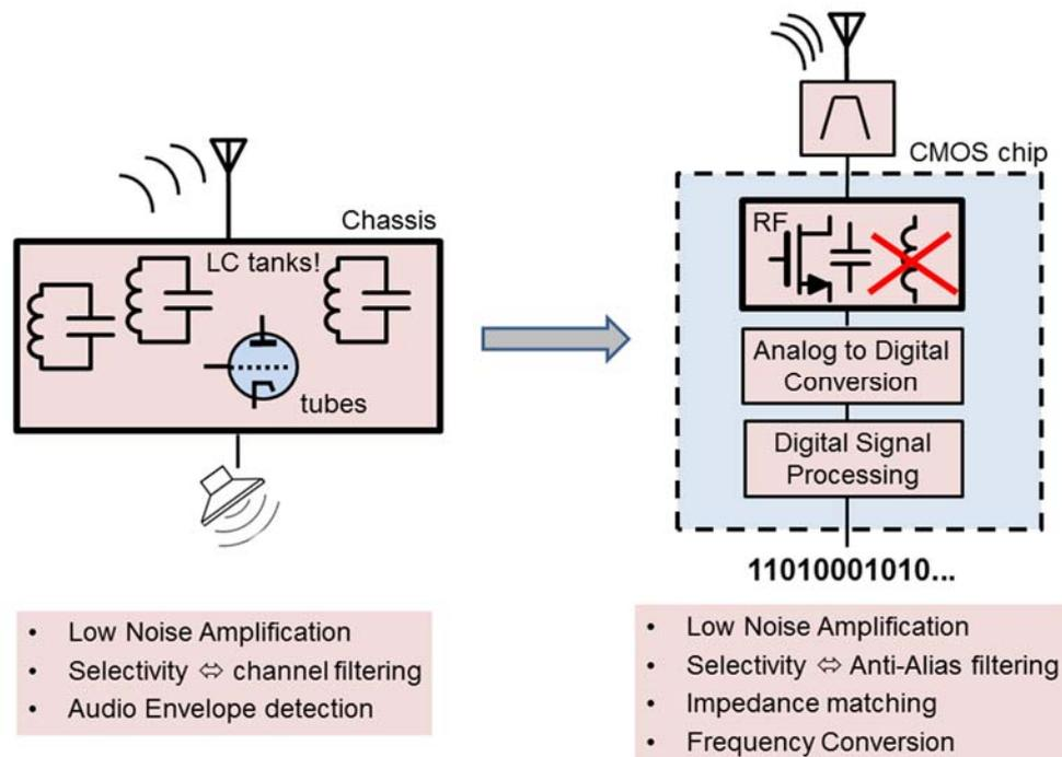
Figure 1: Historical Development of Radio Frequency (RF) receivers during the last century
