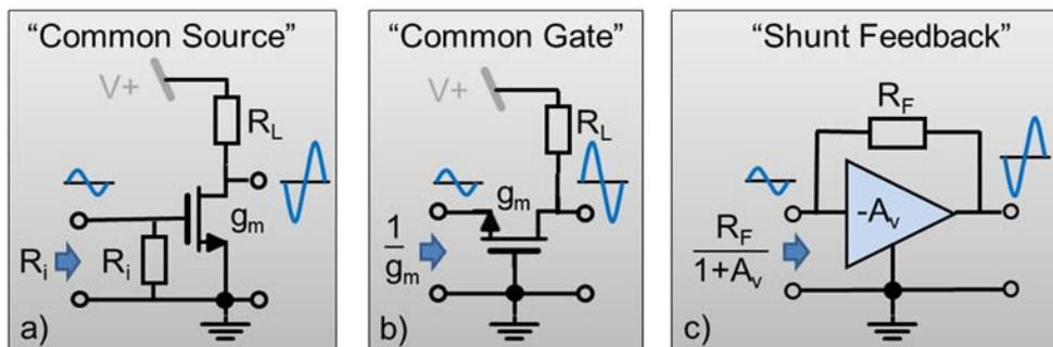
Figure 2: Classical broadband amplifier stages with impedance matching: (a) Common Source with resistor; (b) Common Gate; (c) Shunt feedback stage which can achieve a noise figure <3dB.
