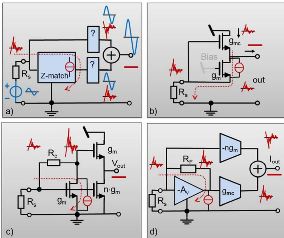
Figure 4: Different Noise Cancelling Circuit Topologies: (a) General concept (b) Original topology discovered by systematic circuit graph generation [2, 3]; (c) First Noise Cancelling LNA with noise figure  $<3\text{dB}$  [4]; (d) Current-output noise cancelling [6].
