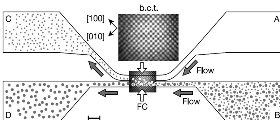
**Figure 4.** Continuous flow particle fractionation using a 3-D array of optical traps (in a body-centred tetragonal lattice = b.c.t.) in a fractionation chamber (FC). Continuous laminar flow is maintained from reservoir A to C and from reservoir B to D. Trap array selectively pushes one species from the mixture in B into the upper flow field, separating it from the other species. Reprinted from [16], with permission.
