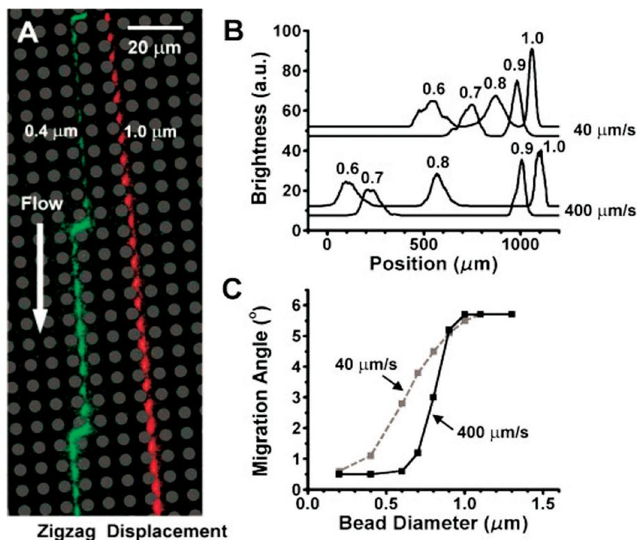
**Figure 3.** Continuous particle sieve employing an obstacle array as shown in Fig. 2. (A) Polystyrene beads (400 nm) move straight down, while 1  $\mu\text{m}$  particles deviate; (B) separation of four different sizes of beads; (C) crucially separation improves with flow speed since separation depends on viscous sorting and not on diffusion. Reprinted from [12], with permission.
