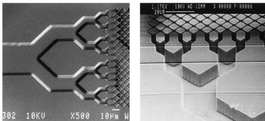
**Figure 1.** Micromachined COMOSS packings for on-chip HPLC and CEC. Reprinted from [5], with permission.
