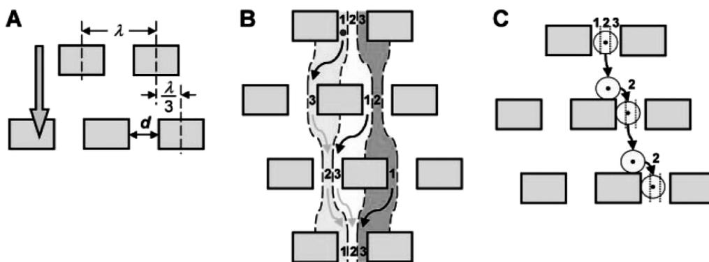
**Figure 2.** Continuous particle sieve. Principle of operation: (A) Design: a row of obstacles, gradually shifted in the flow direction; (B) small particles will move with the flow lines and would not be displaced horizontally; (C) particles with a size in the order of the gap will be continuously displaced. Reprinted from [12], with permission.
