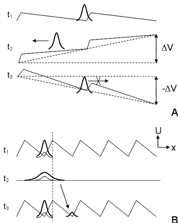
**Figure 5.** Two types of 1-D ratchet devices. (A) Rectifying ratchet, employing an asymmetric potential profile  $U$  rectifying an oscillating net-zero force  $F(t) = -dV/dx$ , where  $-dV/dx$  is an applied potential gradient; (B) Brownian ratchet, employing a time-varying asymmetric potential profile to rectify Brownian motion (Gaussian distribution curves of a slow and fast diffusing species are drawn);  $t_1$ ,  $t_2$  and  $t_3$  denote consecutive moments in time.
