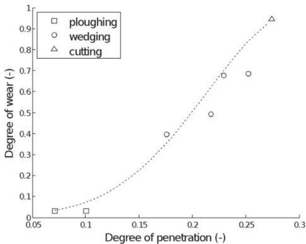
Figure 11. Simulation results; degree of wear plotted against the indentation depth.
