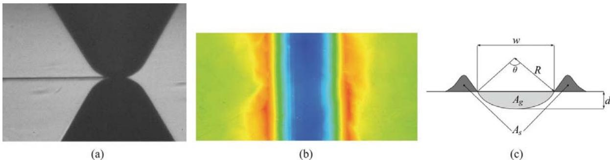
**Figure 5.** Example of a groove resulting from a single asperity scratch test (a) during the experiment and (b) result of a confocal microscope height profile measurement (blue is low, red is high). (c) Schematic illustration of the cross section of a wear scar.
