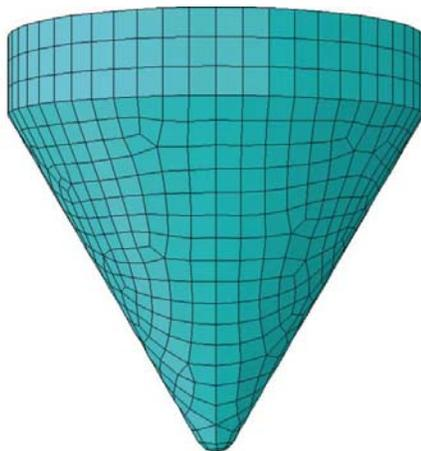
Figure 1. Representation of the tip used in the numerical simulations; spherical  $R = 50 \mu\text{m}$ .
