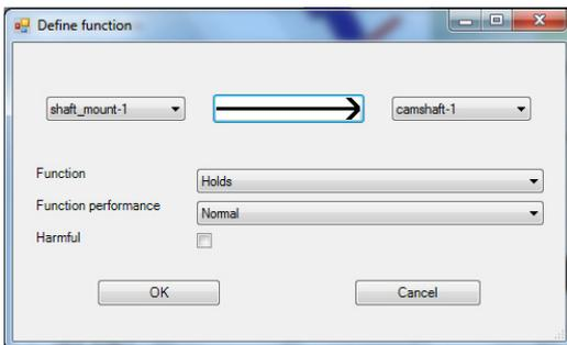
Define function dialog box showing 'shaft\_mount-1' and 'camshaft-1' selected in dropdowns. The function is set to 'Holds', performance is 'Normal', and 'Harmful' is unchecked. Buttons for 'OK' and 'Cancel' are visible.
