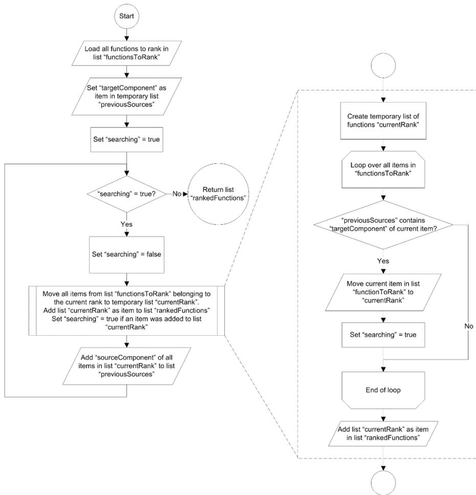
Fig. 8. Flowchart of the function ranking algorithm.
