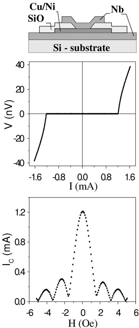
FIG. 2. (Top) Schematic cross section of the sample. (Center) Typical  $I$ - $V$  characteristic. (Bottom) Magnetic field dependence of the critical current  $I_c$  for the junction with  $\text{Cu}_{0.5}\text{Ni}_{0.5}$  and  $d_F = 14$  nm.
