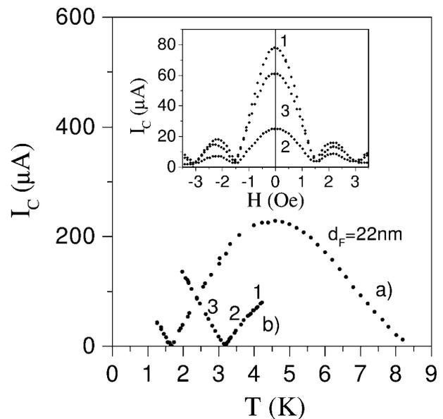
FIG. 3. Critical current  $I_c$  as a function of temperature  $T$  for two junctions with  $\text{Cu}_{0.48}\text{Ni}_{0.52}$  and  $d_F = 22$  nm [17]. Inset:  $I_c$  versus magnetic field  $H$  for the temperatures around the crossover to the  $\pi$  state as indicated on curve b: (1)  $T = 4.19$  K, (2)  $T = 3.45$  K, (3)  $T = 2.61$  K.
