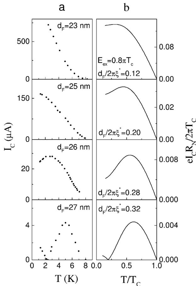
FIG. 4. (a) Critical current  $I_c$  as a function of temperature for  $\text{Cu}_{0.48}\text{Ni}_{0.52}$  junctions with different  $F$ -layer thicknesses between 23 and 27 nm as indicated. (b) Model calculations of the temperature dependence of the critical current in a SFS junction for  $E_{\text{ex}} = 0.8\pi T_c$  and various ratios of  $d_F/2\pi\xi^*$ , where  $\xi^* = \sqrt{\hbar D}/(2\pi k_B T_c)$ .
