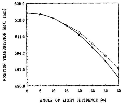
FIG. 3. Position of the passband of the dielectric bandpass filters for *p* and *s* polarization as a function of tilting angle  $\alpha$  ( $\circ$  *p*-polarized light;  $\bullet$  *s*-polarized light).
