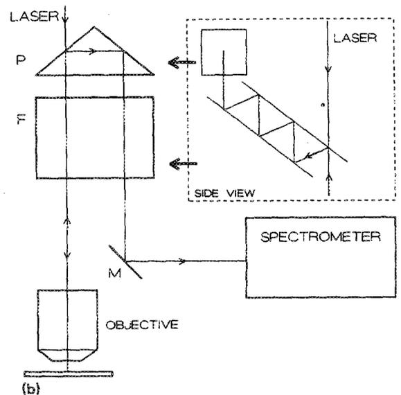
FIG. 4. Two setup configurations employing the RNF set. Abbreviations: *F*: RNF-set, *B*: beamsplitter, *M*: mirror, *P*: prism. (A) RNF set replaces another filter stage. (B) RNF set replaces another filter stage and couples microscope and spectrometer.
