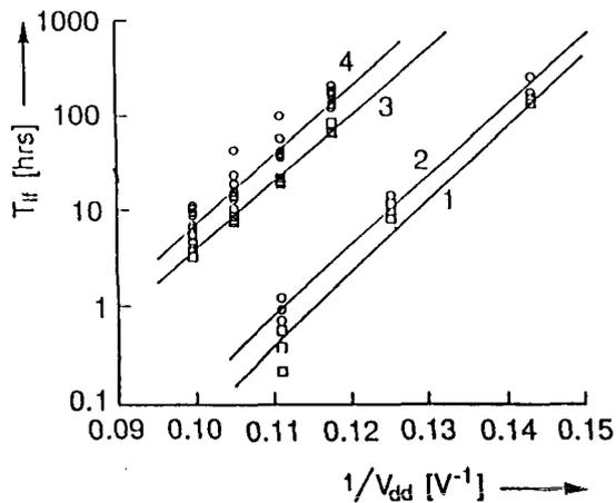
Figure 7. Comparison of hot-carrier lifetime in transistors (curve 1 and 2) and in SRAM products (curve 3 and 4)<sup>12</sup>
