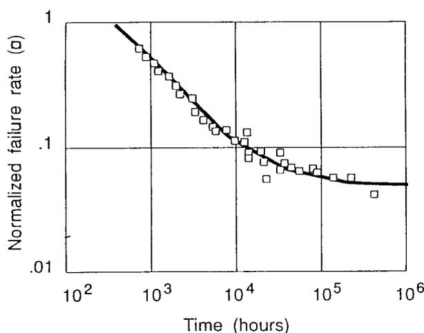
Figure 2. Measured failure rates for a large number of integrated circuits made in bipolar and MOS technology<sup>3</sup>
