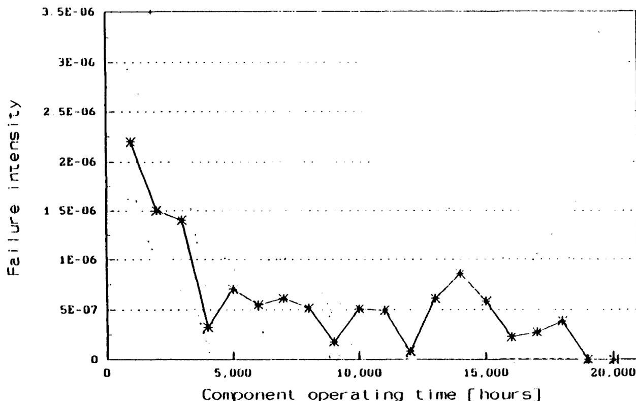
Figure 3. Failure intensity curve for digital MOS ICs with  $10^3$  to  $10^4$  gates
