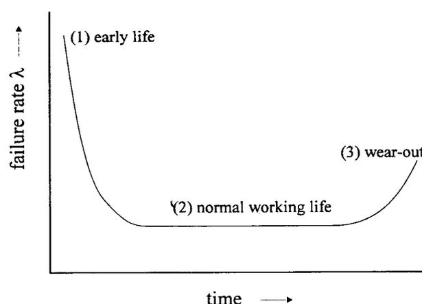
Figure 1. Bathtub curve showing the three most important failure rate phases of a product during its lifetime: (1) early failures (infant mortality), (2) normal operating life and (3) wear-out
