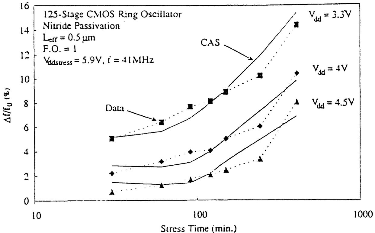
Figure 6. 125-stage CMOS ring oscillator. Measured and (BERT-CAS) simulated frequency decrease at three frequency measuring  $V_{dd}$  values<sup>1</sup>
