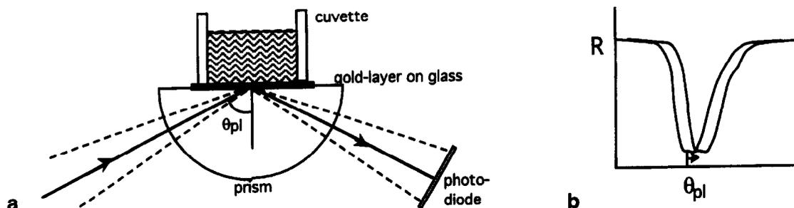
**Figure 1** a, The sensor unit of the SPR apparatus. b, The reflection minimum observed at plasmon angle  $\theta_{pl}$  shifts to a higher value, when for instance, proteins are adsorbed on the gold layer. The actual apparatus, which combines a cylindrical prism and a vibrating mirror, has been described previously<sup>5,6</sup>.
