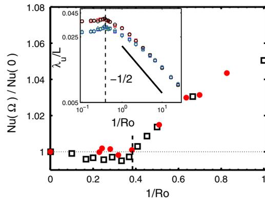
FIG. 2 (color online).  $Nu(\Omega)/Nu(\Omega = 0)$  for  $Ra = 2.73 \times 10^8$  and  $Pr = 6.26$ . Red solid circles: experimental data ( $T_m = 24^\circ\text{C}$  and  $\Delta = 1.00\text{ K}$ ). Open black squares: numerical results. The experimental error coincides approximately with the symbol size, and the numerical error is approximately 0.5%. Inset: Thickness of the kinetic BL. For dashed vertical lines and inset, see Fig. 1.
