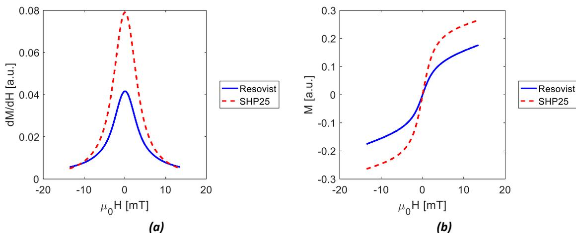
Figure – SPaQ results, measured on Resovist (Bayer Schering Pharma GmbH) and SHP-25 (Ocean Nanotech) samples containing 750  $\mu\text{g}$  iron in a total volume of 150  $\mu\text{l}$ , at a frequency of 2.5 kHz. (b) is a numerical integration of (a).
