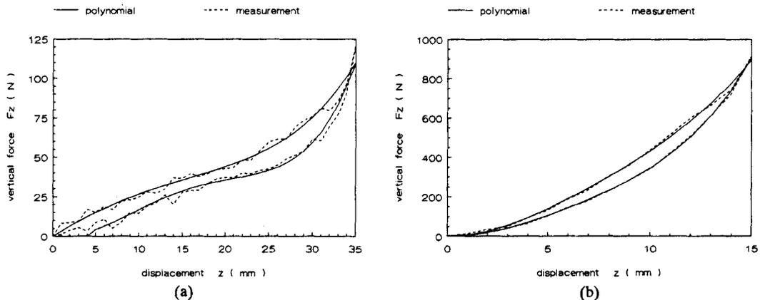
Fig. 2. Typical load-displacement curves showing the hardening spring behaviour. Auxiliary is the best fitted polynomial according to the least square method. The depicted measurements are heel strike (a) and toe-off (b) from the Hanger Quantum foot without shoe.
