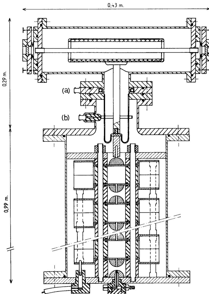
Fig. 1. Cross-section of the laser construction and Marx generator (a): Rogowski coil, (b): Capacitive coupled differentiating voltage sensor.
