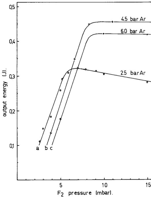
Fig. 3. Output energy as a function of the F<sub>2</sub> pressure at argon pressures of 2.5 bar (a), 4.5 bar (b) and 6 bar (c). Krypton pressure 150 mbar, current density 375 A/cm<sup>2</sup>.
