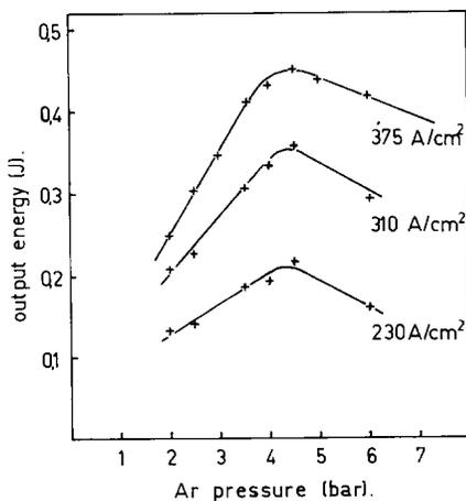
Fig. 4. Dependence of output energy on argon pressure. F<sub>2</sub> pressure: 10 mbar, Kr pressure: 150 mbar. Current densities: 230, 310 and 375 A/cm<sup>2</sup>.
