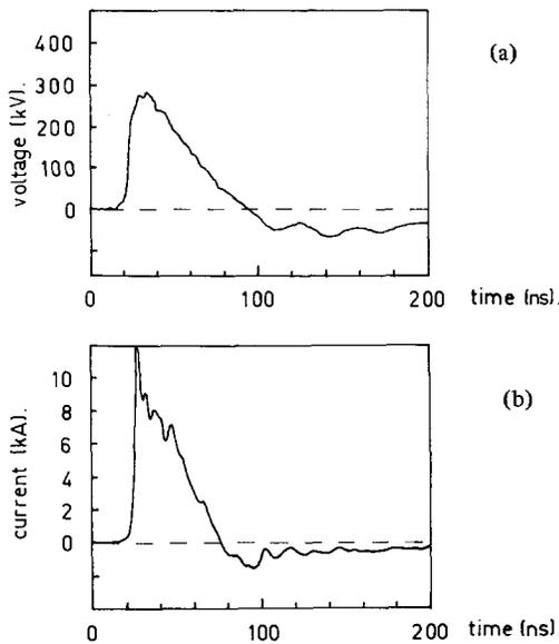
Fig. 2. (a) Voltage pulse and (b) current pulse at vacuum diode as a function of time for a generator charging voltage of 60 kV.
