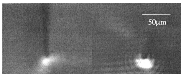
FIG. 2. Mode profiles (633 nm, TE polarization) of two different waveguides written into the bulk of the Ti 3+ :Sapphire sample. (Visible diagonal fringes are due to a detection artifact.)
