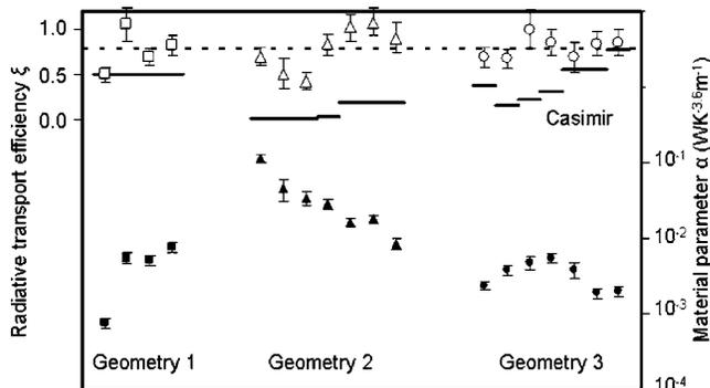
FIG. 3. Thermal data analyzed assuming diffuse phonon transport (filled symbols, right axis) and radiative phonon transport (open symbols, left axis). The dashed line indicates radiative transport with  $\xi = 0.78$ ; the horizontal lines indicate the Casimir limit to  $\xi$ . The data of Geometry 2 are arranged in order of decreasing membrane dimensions starting from  $4000 \mu\text{m}$  (left) down to  $440 \mu\text{m}$  (right).
