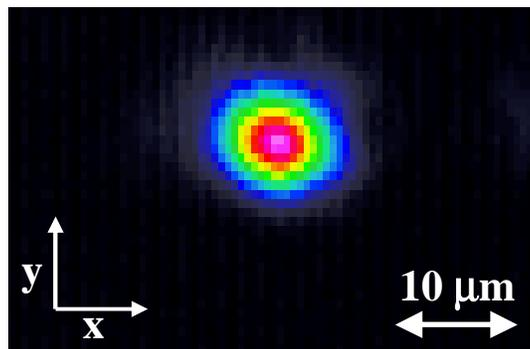
Fig. 4. Laser mode profile obtained from a Ti:sapphire rib waveguide of height  $3.5\ \mu\text{m}$  and width  $10\ \mu\text{m}$  using a 4.6% output coupler at an absorbed power of 350 mW.
