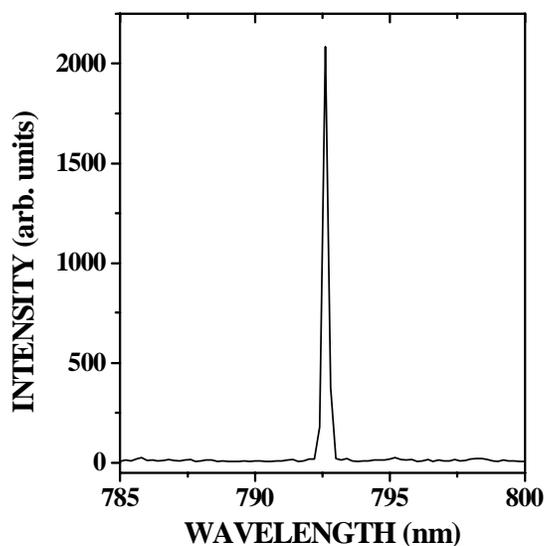
Fig. 2. Lasing spectrum originating from a Ti:sapphire rib waveguide for an absorbed pump power of 350 mW. The structure was 3.5  $\mu\text{m}$  and 10  $\mu\text{m}$  in height and width, respectively.
