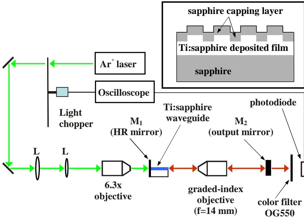
Fig. 1. Experimental configuration for the investigation of the rib waveguide lasers. The laser cavity is formed by the mirrors  $M_1$  and  $M_2$ . The geometry of the resulting structure after the fabrication process is shown in the inset.
