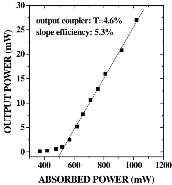
Fig. 3. Output power from a rib waveguide laser with height and width of  $3.5\ \mu\text{m}$  and  $10\ \mu\text{m}$ , respectively, as a function of the absorbed power for an output coupler with a 4.6% transmission at the lasing wavelength
