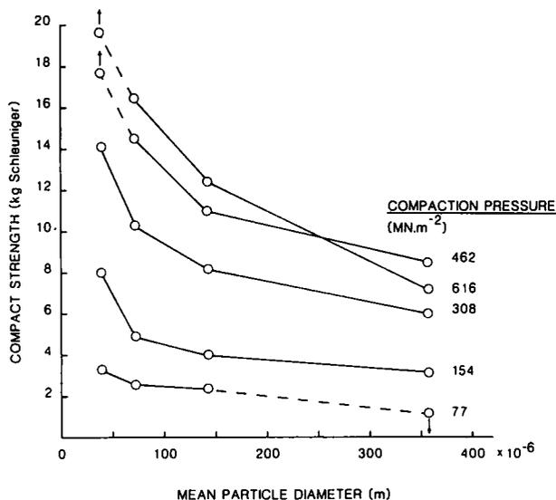
FIGURE 1 Compact strength versus mean original particle diameter for tablets compressed from sieve fractions of crystalline  $\alpha$ -lactose monohydrate at different compaction pressure levels ( $n = 10$  for each point)
