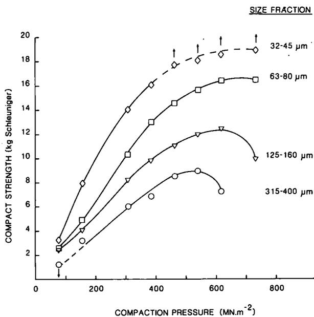
FIGURE 2 Comparison of compact strength versus applied compaction load for tablets from sieve fractions of crystalline  $\alpha$ -lactose monohydrate
