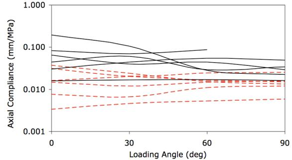
**Figure 2:** Axial tensile compliance of the cement-bone interface as a function of loading angle for postmortem (solid black lines) and laboratory prepared specimens (dashed red lines).
