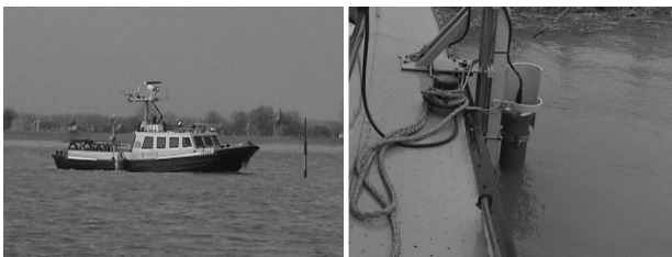
Figure 8. The used research vessel for flow measurements in the Rhine River in November 1998 (left). The picture on the right shows the attached ADCP (pictures: aqua vision).
