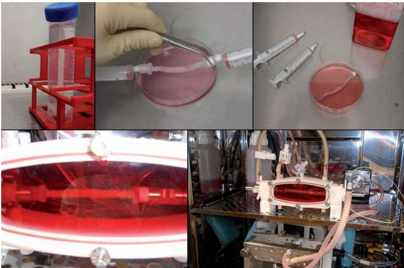
**Figure 2.** Overview of vascular tissue engineering. From left to right and top to bottom: tubular PTMC scaffold, SMC seeding, SMC-containing construct, construct in flow chamber, pulsatile flow bioreactor.
