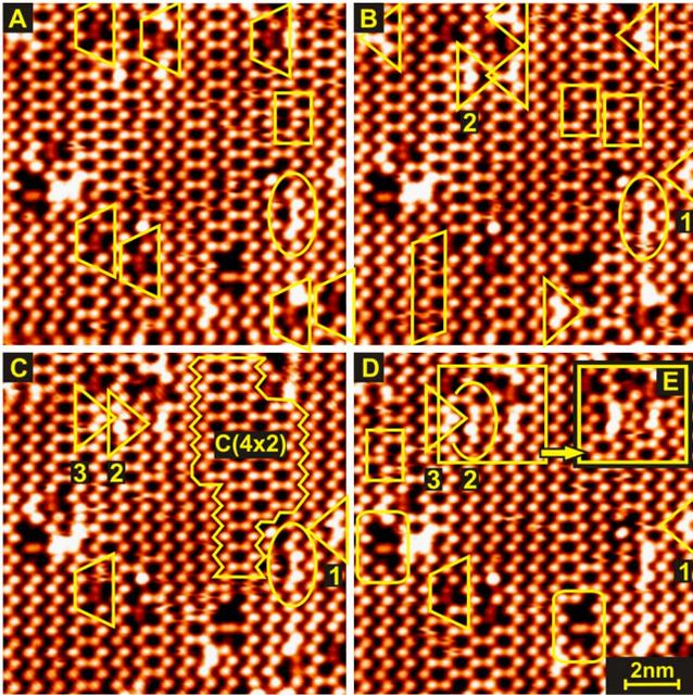
FIG. 1. (Color online) Five successive STM images of a Ge(001) surface—including inset E—recorded at 77 K, after exposure to 100 L hydrogen. Tunnel current 0.5 nA is and sample bias  $-1.0$  V. The time lapse between successive images is 5 min.
