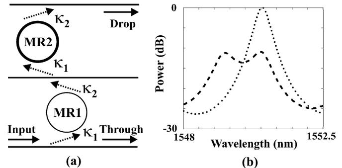
Fig. 1. (a) Schematic drawing of a switch based on two MRs and (b) simulated responses of switch in ON-state (dotted line) and switch in OFF-state (dashed line).
