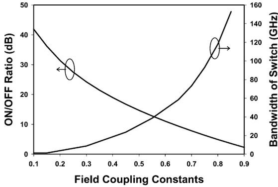
Fig. 2. Effect of coupling constants on the ON–OFF ratio of the switch and the 3-dB bandwidth of the switch. Both the coupling constants are assumed equal, ring losses of 5 dB/cm and a radius of 50  $\mu\text{m}$ .
