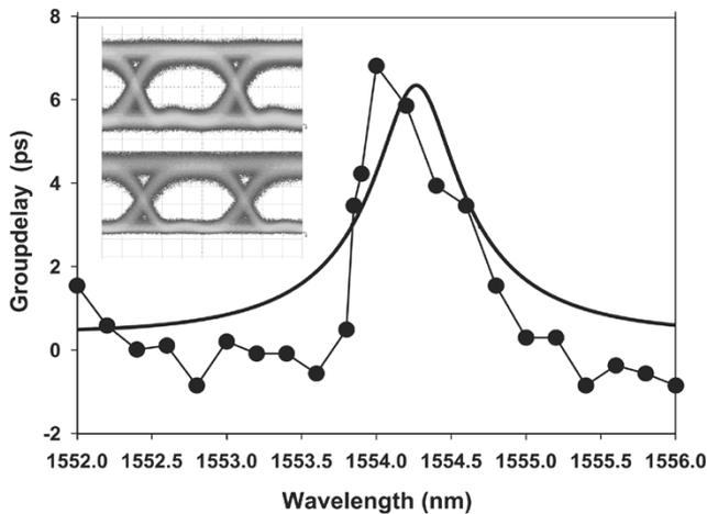
Fig. 5. Measured and simulated group delay of a single ring. Also shown are the eye diagrams of 10-Gb/s NRZ signals of modulator output (top) and after being filtered by an MR (bottom).
