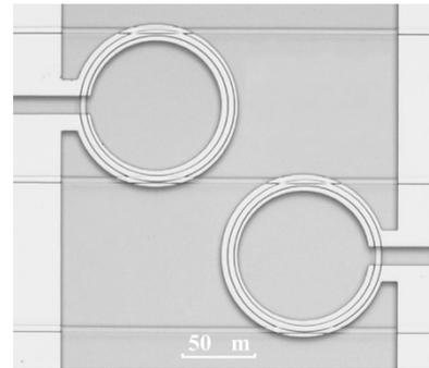
Fig. 4. Microscope photograph of a realized switch based on two MRs.
