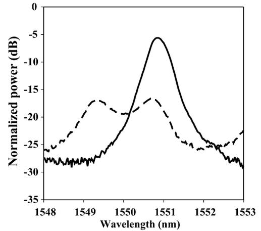
Fig. 3. Measured response of switch. Solid line: ON-state. Dashed line: OFF-state.
