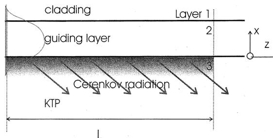
Fig. 1. Schematic picture of the considered three-layer system.
