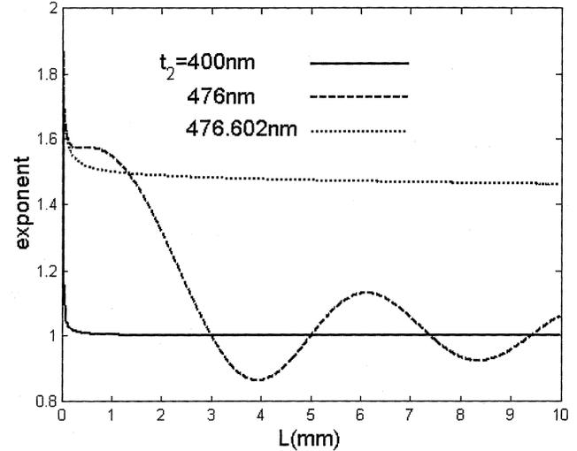
Fig. 5. Numerically evaluated exponent of  $L$  occurring in the length dependence of the conversion efficiency,  $\eta$  as a function of  $L$ . Parameters, except the thickness of the guiding layer are given in Table I.
