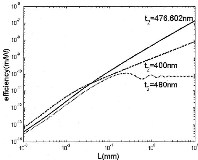
Fig. 6. Calculated conversion efficiencies,  $\eta(L)$ , according to (17) for the structure given in Table I, for various values of the thickness of the guiding layer.
