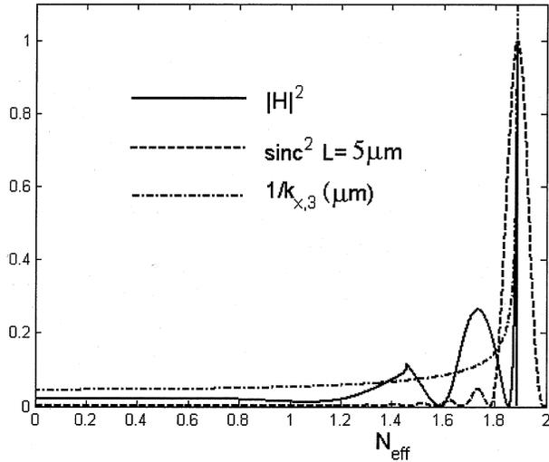
Fig. 3. Calculated values of  $1/k_{x,3}$ ,  $|H|^2$  and the  $\text{sinc}^2$ -function for  $L = 5 \mu\text{m}$  defined in (15) as a function of  $N_{eff} (\equiv k_z/k_0)$ . The parameters are according to Table I.
