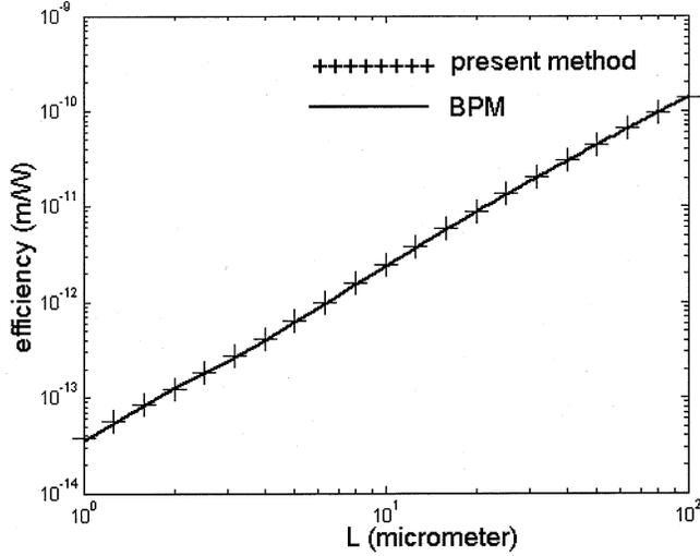
Fig. 2. Comparison of calculations of the conversion efficiency according to the present method with those according to BPM. The parameters are given in Table I.
