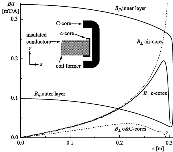
Fig. 2. Magnetic field as a function of the axial position ( $z = 0$ , midplane) in a coil with ferromagnetic elements to reduce the  $B_{\perp}$  component. Coil edge with small and large ferromagnetic cores.
