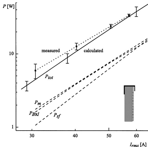
Fig. 5. Measured and calculated loss of the model coil with c-cores as a function of current through the coil. ( $f = 48$  Hz,  $T = 77$  K).
