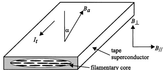
Fig. 1. Tape superconductor and the definitions of  $B_a$ ,  $\alpha$ ,  $I_t$  and the directions  $B_{\perp}$  and  $B_{\parallel}$ .
