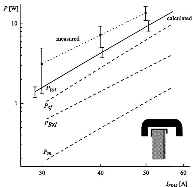
Fig. 6. Measured and calculated loss of the model coil with c and C-cores as a function of current through the coil. ( $f = 48$  Hz,  $T = 77$  K).
