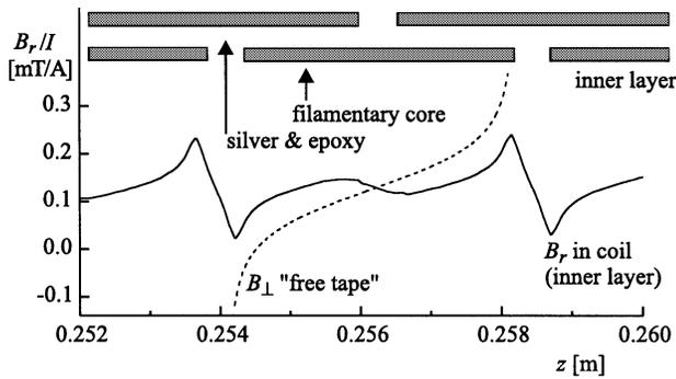
Fig. 3. Magnetic field detail, calculated in a model with separate filamentary cores. Comparison with field in a free tape (field of the tape plus the average of the field in the coil over one tape width).
