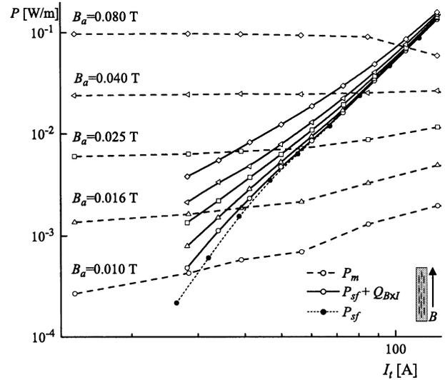
Fig. 4. AC loss components of a BSCCO/Ag tape conductor carrying AC transport current and exposed to AC magnetic field parallel to the wide face of the tape. The symbols represent measured points, the lines are guides to the eye. ( $f = 48$  Hz,  $T = 77$  K).
