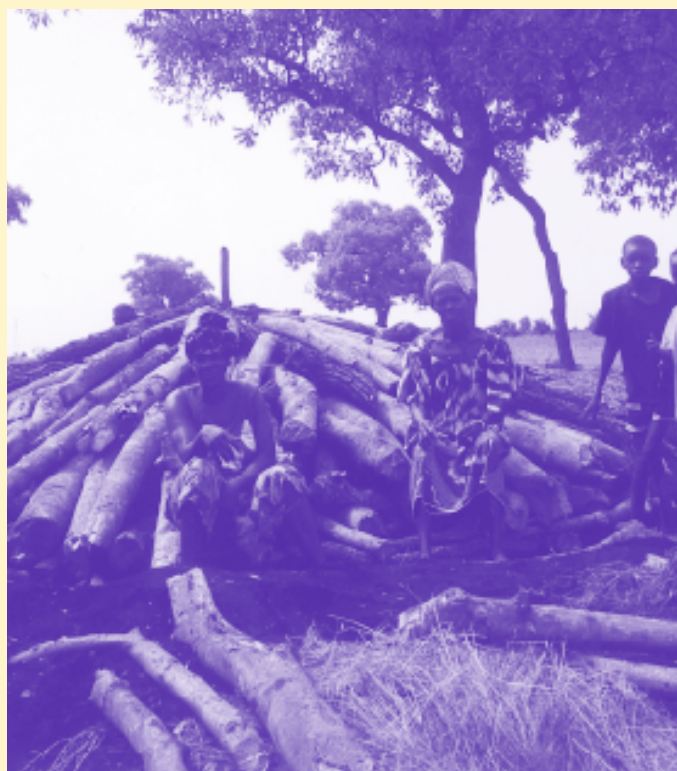
Djénéba Diarra (right) sitting on a half constructed Casamance Kiln. (Photo: Courtesy of Margaret Skutsch)
