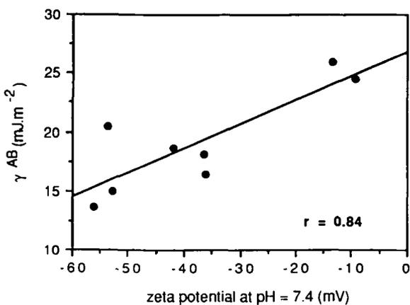
Fig. 3. Relation between the acid/base component of the surface free energy of the eight *E. coli* strains based on the concept of Lifshitz-van der Waals and acid/base surface free energy components (17,18), and the zeta potentials at pH = 7.4.
