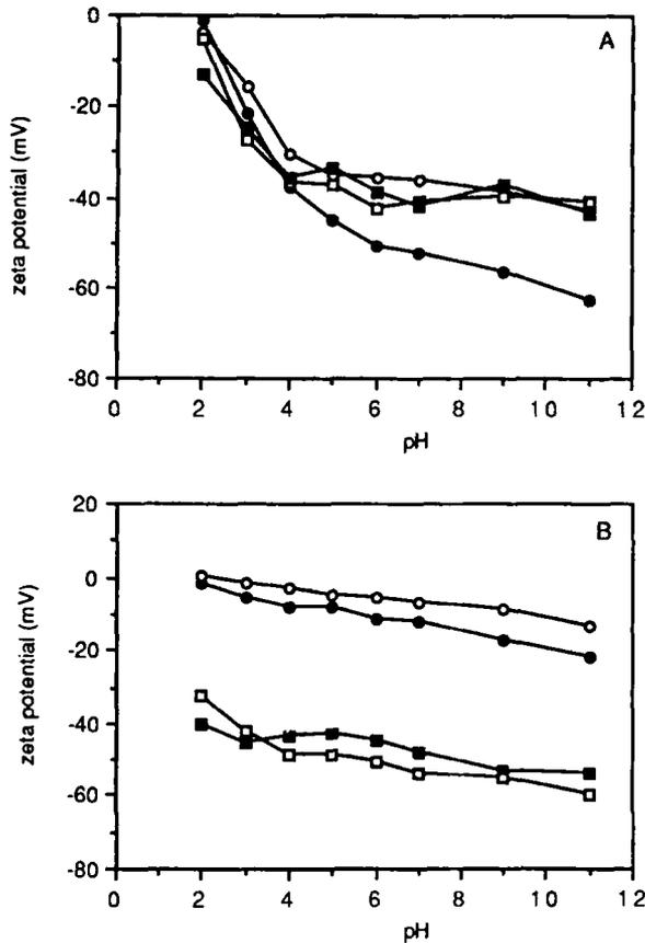
Fig. 1. Zeta potentials as function of the pH. Electrophoretic mobility was measured in 0.01M KCl buffered with  $10^{-3}$ M phosphate. The pH was adjusted with 1M aqueous KOH and HCl solution in water. A: group one, containing strains O8K(A)28, O161K-, O2K7, and O39K1. B: group two, containing strains O2K2 and O83K?; group three, containing strains O111K58 and O157K-. A. —○— O8K(A)28; —●— O161K-; —□— O2K7; —■— O39K1. B. —○— O111K58; —●— O157K-; —□— O83K?; —■— O2K2.
