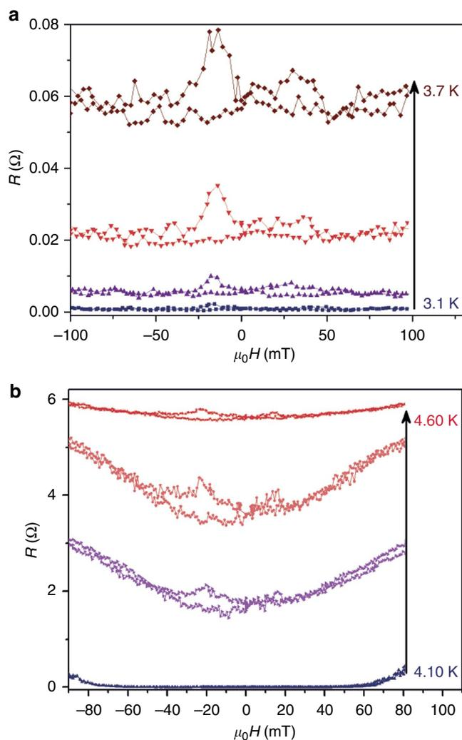
**Figure 3 | Resistance-field measurements for different spin-mixer layer thicknesses.** Four-point resistance measurements of Nb(4 nm)/Py(8 nm)/Ho( $d_{\text{Ho}}$ )/Nb( $d_{\text{Nb}}$ )/Ho( $d_{\text{Ho}}$ )/Py(5 nm)/FeMn(5 nm) spin valves in the superconducting transition. **(a)**  $R$ - $H$  for 2-nm-thick top and bottom Ho layers and 26-nm-thick Nb layer. **(b)**  $R$ - $H$  for 7-nm-thick Ho layers and 26-nm-thick Nb layer.
