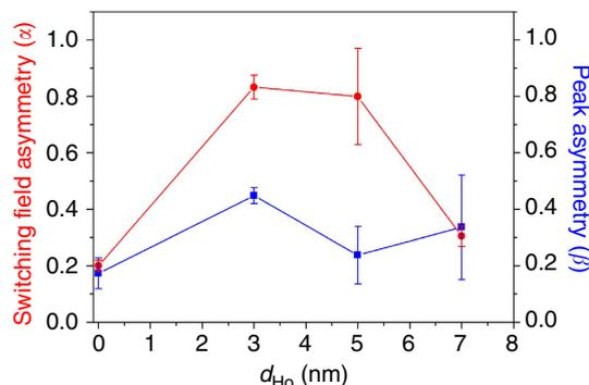
**Figure 4 | Asymmetry in peak widths.** The switching field asymmetry calculated from the  $M$ - $H$  loops ( $\alpha$ ) and the peak asymmetry from  $R$ - $H$  ( $\beta$ ) are plotted as a function of Ho thickness. The error bars represent 1 s.d. on each side.
