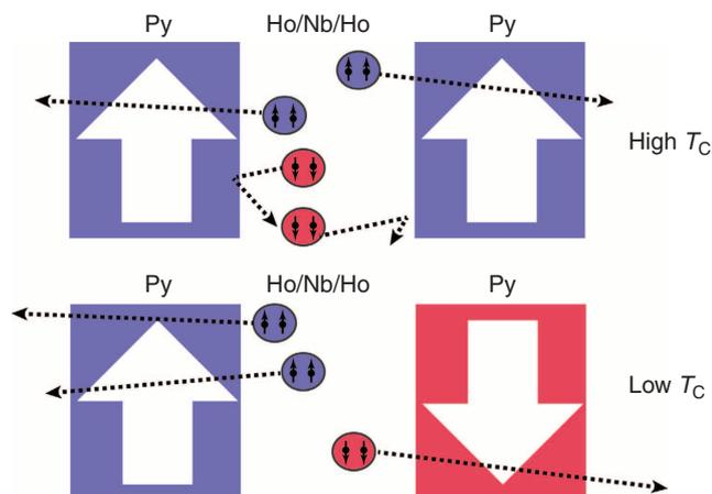
**Figure 5 | Illustration of the spin selectivity.** A cartoon illustrating the possible behaviour of spin-one triplet pairs in Py/Ho/Nb/Ho/Py/FeMn F-S-F spin valves in the parallel (top) and antiparallel states (bottom).
