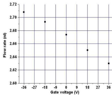
Fig. 9. Change in flow rate (nl) as a function of  $V_G$ .
