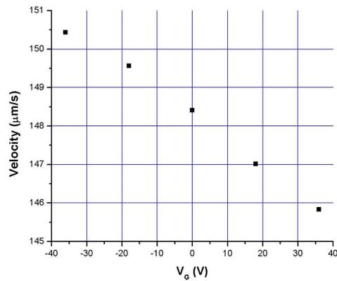
Fig. 8. Uniform velocity at long distance from the gate region.
