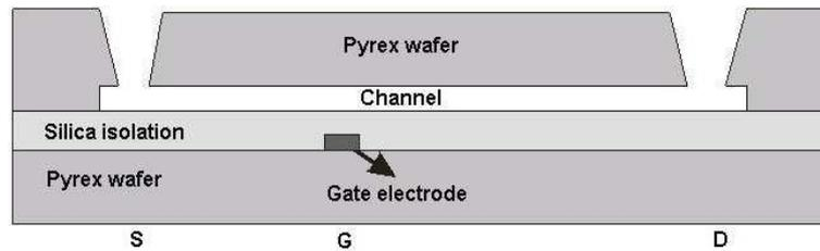
Fig. 1. Schematic longitudinal cross-section of the FlowFET.
