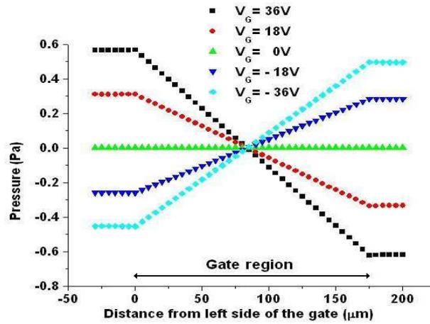
Fig. 7. Pressure variation along the gate region (reference pressure = 0).
