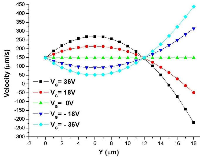
Fig. 3. Velocity distribution corresponding to the middle of the gate, as function of  $V_{Gate}$ .
