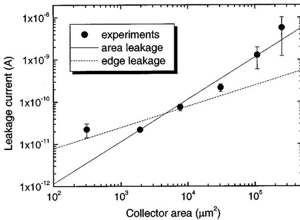
Fig. 6. Dependence of collector leakage current on collector area. The circles are the leakage currents of the reversed biased collector diode (1 V). Two lines that represent leakage current proportional to area (solid) and edge length (dotted) have also been included.
