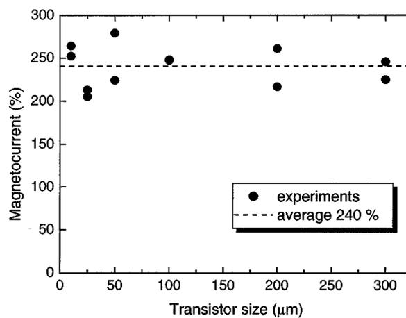
Fig. 4. Dependence of magnetocurrent on transistor size. The dotted line shows the average MC of 240%.
