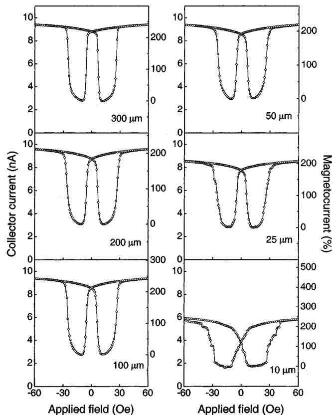
Fig. 3. Collector current as a function of applied field for various sized transistors. The emitter current is set to 1 mA. The absolute collector current is plotted on the left vertical axis and the corresponding MC on the right axis.
