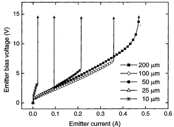
Fig. 7. Emitter bias voltage versus emitter current for different sized SVTs; the abrupt jump indicates the breakdown point.
