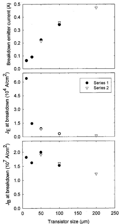
Fig. 9. (Top) Emitter current at device breakdown for two series of SVTs. (Middle) Emitter current density ( $J_E$ ) at device breakdown. (Bottom) Base current density ( $J_B$ ) at device breakdown.
