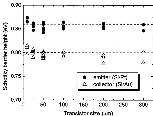
Fig. 2. Schottky barrier height of emitter and collector diode for various transistor sizes. The dotted lines indicate the average barrier height: 0.86 eV for the Si/Pt emitter and 0.80 eV for the Si/Au collector. The transistor size is an edge length of the square emitter.
