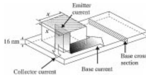
Fig. 8. Schematic diagram of the SVT showing the current flow and the cross sections.  $x$  is 10, 25, 50, 100, or 200  $\mu\text{m}$ .
