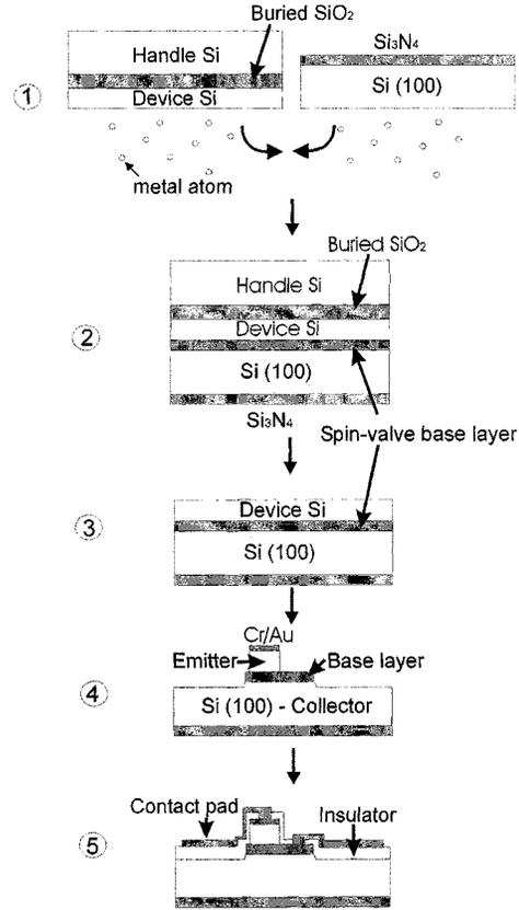
Fig. 1. Schematic diagram of the fabrication process. See text for details.
