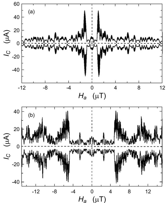
FIG. 3. Critical current  $I_c$  as a function of applied magnetic flux  $H_a$  for (a) an array of eight alternating 0 and  $\pi$  facets of  $25 \mu\text{m}$  width ( $V_{\text{bias}} = 1 \mu\text{V}$ ), and (b) an array of 80 alternating 0 and  $\pi$  facets of  $5 \mu\text{m}$  width ( $V_{\text{bias}} = 5 \mu\text{V}$ ).
