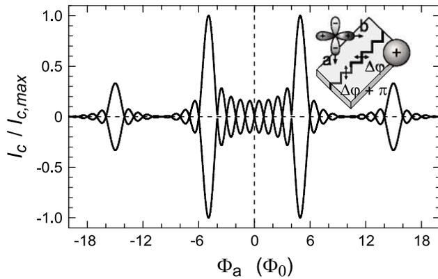
FIG. 1. Calculated magnetic flux dependence of the normalized critical current  $I_c/I_{c,\max}(\Phi_a)$  for an array of ten facets, composed of standard and  $\pi$ -Josephson contacts. The inset shows a schematic of the array, based on  $\text{YBa}_2\text{Cu}_3\text{O}_7/\text{Au}/\text{Nb}$  junctions.
