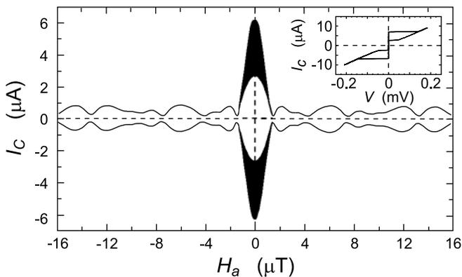
FIG. 2. Critical current  $I_c$  as a function of applied magnetic flux  $H_a$  for a  $50 \mu\text{m}$  wide  $\text{YBa}_2\text{Cu}_3\text{O}_7/\text{Au}/\text{Nb}$  ramp-type junction, for positive and negative bias voltage of  $2.5 \mu\text{V}$ . The dark area indicates the hysteresis in the current-voltage ( $I$ - $V$ ) characteristic. The inset presents an  $I$ - $V$  characteristic for the same junction.
