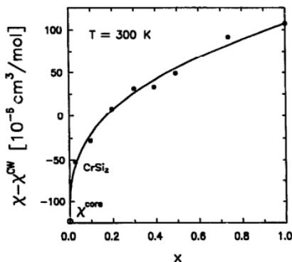
Fig. 7. Experimental (●) and calculated (—) room temperature susceptibilities of  $\text{Cr}_{1-x}\text{V}_x\text{Si}_2$  solid solutions. The experimental room temperature susceptibilities have been corrected for contributions of permanent magnetic moments.
