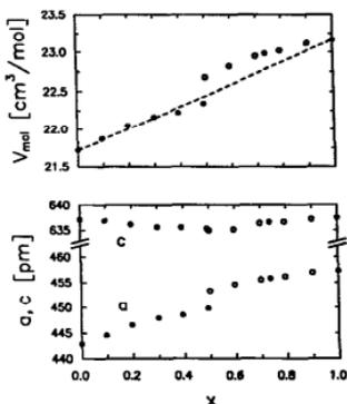
Fig. 1. Lattice parameters and molar volumes of  $\text{Cr}_{1-x}\text{V}_x\text{Si}_2$  solid solutions. The unit cell is hexagonal (C40 structure) and contains three formula units. The dashed line shows the behavior predicted by Vegard's law.
