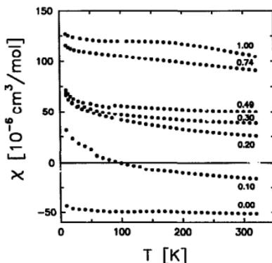
Fig. 4. Temperature dependence of the magnetic susceptibility for  $\text{Cr}_{1-x}\text{V}_x\text{Si}_2$  solid solutions. The data are given in units of the electro-magnetic cgs-system.
