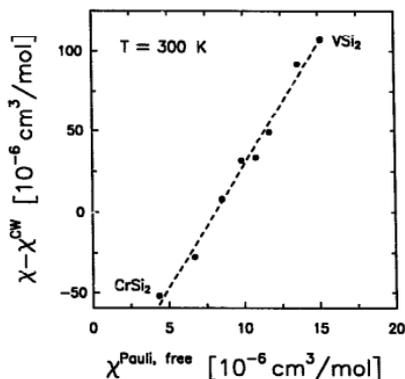
Fig. 6. Experimental room temperature susceptibilities of  $\text{Cr}_{1-x}\text{V}_x\text{Si}_2$  solid solutions corrected for the contributions of permanent magnetic moments and plotted versus the calculated free-electron Pauli susceptibilities of Table 2. The dashed line represents a linear fit  $y = a + bx$  with an intercept of  $-123 \times 10^{-6} \text{ cm}^3 \text{ mol}^{-1}$  and a slope of 15.2.
