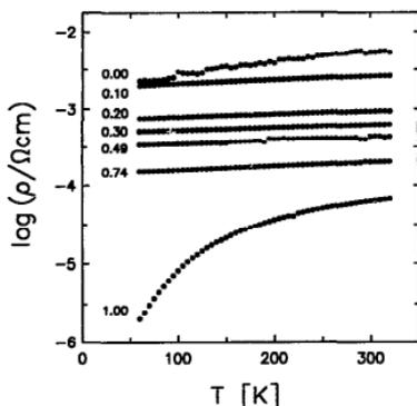
Fig. 2. Temperature dependence of the resistivity for  $\text{Cr}_{1-x}\text{V}_x\text{Si}_2$  solid solutions in a semi-logarithmic plot.
