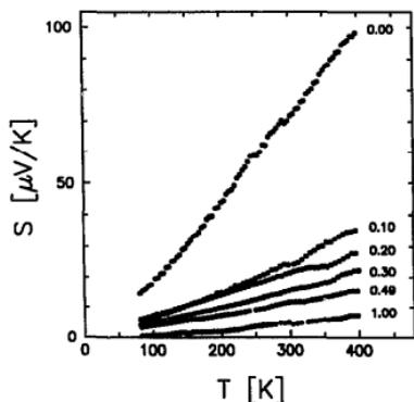
Fig. 3. Temperature dependence of the thermopower for  $\text{Cr}_{1-x}\text{V}_x\text{Si}_2$  solid solutions.
