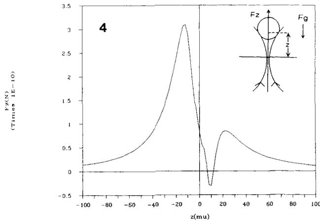
FIG. 3. Calculated values of the radiation force  $f(z)$  on a sphere as a function of  $z$  for different relative refractive indices; radius of the sphere =  $3.75 \mu\text{m}$  and radius of the beam waist at the focus =  $1.8 \mu\text{m}$ .
