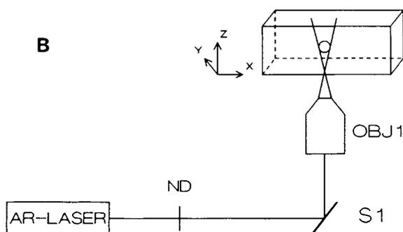
FIG. 6B. Schematic drawing of the configuration used: gravity trap (seen from aside); the cuvet can be moved in X, Y, and Z direction. AR-Laser, Argon laser ( $\lambda = 488 \text{ nm}$ ); ND, neutral density filter; S1, mirror; OBJ, objective.
