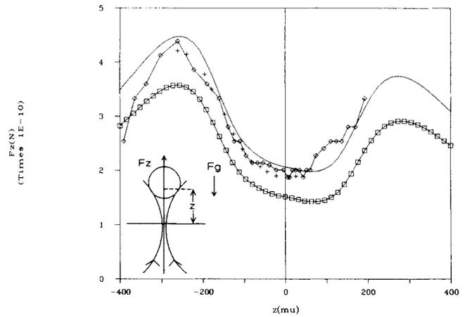
FIG. 8. Measurements of  $f(z)$  as a function of  $z$  relative to the calculated values for spheres with a radius of  $16 \mu\text{m}$  and a focus with a radius of  $1.8 \mu\text{m}$ . Solid line with squares, calculated values for a refractive index of the sphere = 1.60. Solid line, calculated values for refractive index of the sphere = 1.65. Line with rhombs, dynamic measurements. Crosses, static measurements.
