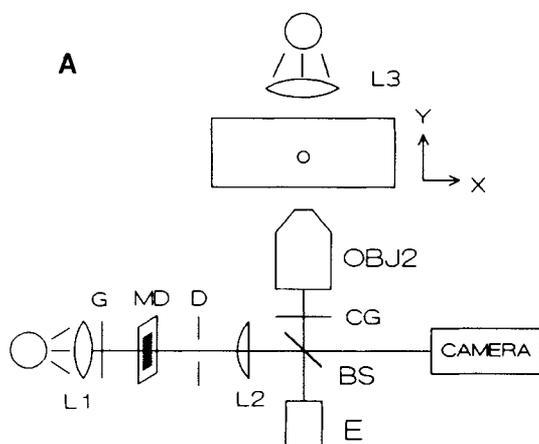
FIG. 6A. Schematic drawing of the configuration used: measuring system (seen from above). L, lens; OBJ, objective; G, ground glass; MD, millimeter division; D, diaphragm; BS, beam splitter; CG, color glass; E, eyepiece.
