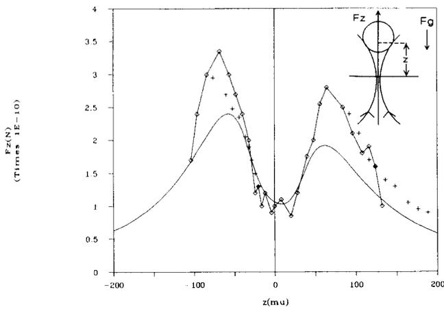
FIG. 7. Measurements of  $f(z)$  as a function of  $z$  relative to the calculated values for spheres with a radius of  $3.75 \mu\text{m}$  and a focus with a radius of  $1.8 \mu\text{m}$ . Solid line, calculated values for a refractive index of the sphere = 1.54. Line with rhombs, dynamic measurements. Crosses, static measurements.
