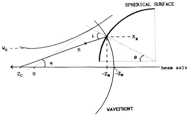
FIG. 2. Determination of the angle  $\alpha$  between the beam axis and the ray of a gaussian laser beam that hits the point  $M(X_M, Z_M)$  of a spherical surface.  $R$  is the radius of the spherical wave front,  $Z_C$  is the point from which the ray seems to come, assuming that the ray is orthogonal to the wave front, and  $w_0$  is the beam waist at the focus (at  $z = 0$ ).
