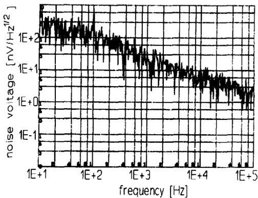
Figure 3 Measured voltage noise of the pyroelectric sensor element for  $R_{\text{bias}} = 1 \text{ M}\Omega$  as a function of the frequency.
