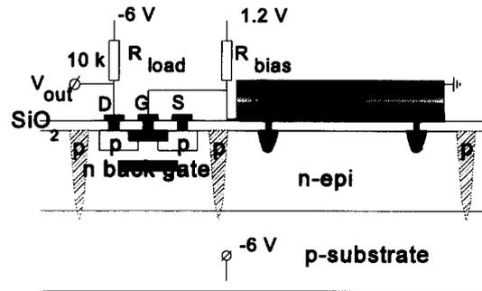
Figure 1 Vertical cross-section of the layout of a single pyroelectric sensor.
