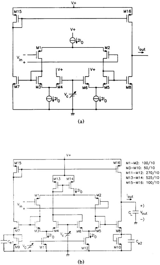
Fig. 1. (a) OTA proposed in [9]. (b) Modified OTA using stacked square-law transistors.
