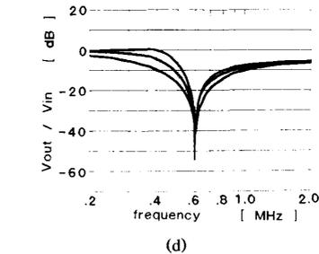
Fig. 3. (a) Second-order notch filter. (b) Frequency characteristics of the filter for  $V_0$  tracking  $V_c$  according to  $(V_c - V_{Teq})/(V_0 - V_T) = 3.2$ . (c) Idem for a constant  $V_0 = 0.64$  V. (d) Idem for constant  $G_{m1}G_{m2}$  and  $Q = 0.5$ ,  $Q = 1$ , and  $Q = 2$ .
