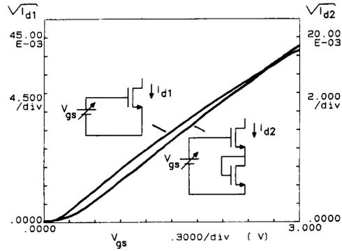
Fig. 2.  $\sqrt{I_d}$  versus  $V_{gs}$  of a single 50/10 NMOS transistor compared to a stacked pair of 50/10 NMOS transistors: the stacked pair has a better square-law behavior for  $V_{gs} = 0.6-3$  V.
