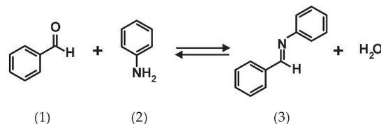
Fig. 5 Imine (3) formation from benzaldehyde (1) and aniline (2).
