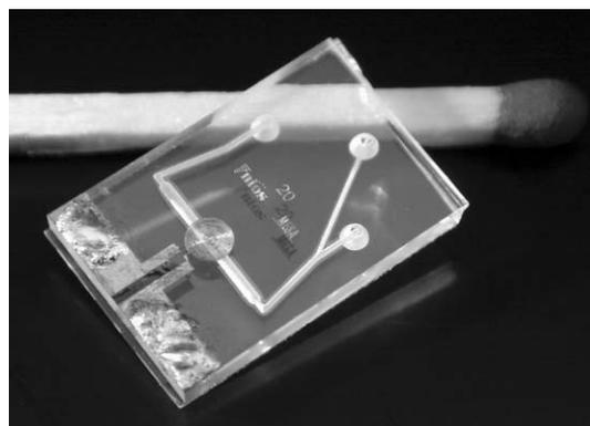
**Fig. 3** The glass NMR chip with planar micro coil. Chip size is 1 by 1.5 cm; channel width underneath coil is 500  $\mu\text{m}$ .
