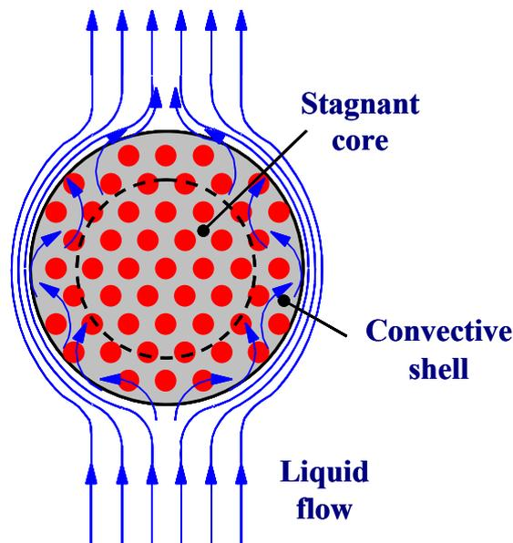
**Figure 1.** Liquid flow around and through a textile yarn.
