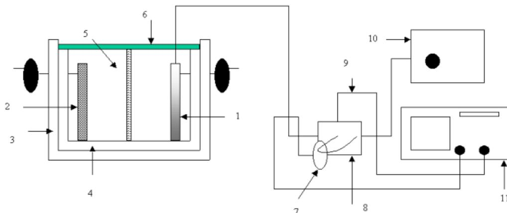
**Figure 3.** Experimental set-up: 1- Sonicator plate, 2 - Reflector, 3 - Thermal insulation of the bath, 4 - Absorbent rubber lining, 5 - Frame for the textile, 6 - Sliding bar, 7 - Current clamp, 8 - Voltage current monitoring box, 9 - Voltage probe, 10 - Ultrasound amplifier, 11 - Digital oscilloscope.
