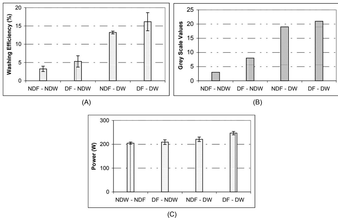
**Figure 6.** (A) Cleaning efficiency in different sets of experiments. (B) Average standard deviation in the grey scale values of the pixels in the images of the different samples of different sets. (C) Power consumption of the bath in different sets of experiments.
