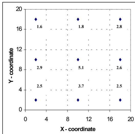
**Figure 4.** Distribution of the acoustic pressure amplitudes (bar) at different locations in the plane of cleaning experiments between the sonicator plate and the reflector at a distance of 2.5 cm from the sonicator plate.
