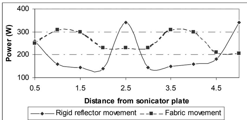
**Figure 5.** Variation in the power consumption of the bath with reflector movement in front of the sonicator plate, and as a function of textile movement between the sonicator plate and the reflector.
