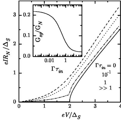
FIG. 8.  $IV$  characteristics at  $k_B T / \Delta_S = 0.25$  and  $\gamma_{\text{eff}} \gg 1$  on the basis of Eq. (48) for several values of the inelastic scattering parameter  $\Gamma \tau_{in}$ . The inset shows the subgap conductance at  $eV = \Delta$  as a function of  $\Gamma \tau_{in}$ .
