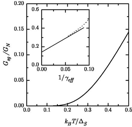
FIG. 4. Normalized conductance at  $eV = \Delta_S$  as a function of temperature (normalized to  $\Delta_S$ ) for  $\gamma_{\text{eff}} \gg 1$ . The inset shows the normalized conductance at  $eV = \Delta_S$  as a function of  $1/\gamma_{\text{eff}}$  at  $k_B T / \Delta_S = 0.5$ .
