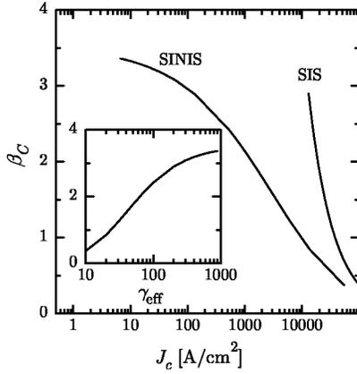
FIG. 12. Theoretical model for  $\beta_C$  as function of  $J_c$  (and as function of  $\gamma_{\text{eff}}$  in the inset), based on the contribution of Andreev channels to the subgap conductance in high- $J_c$  junctions at  $T=4.2$  K, in comparison with the hysteresis of SIS junctions.
