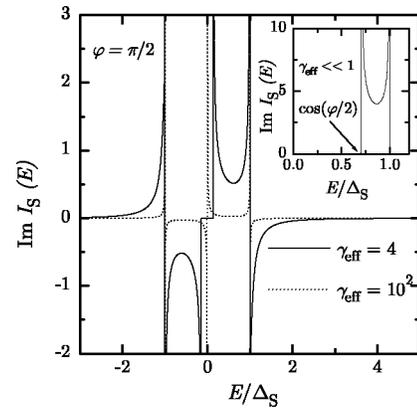
FIG. 3. Normalized spectral supercurrent density as a function of energy for various values of the suppression parameter  $\gamma_{\text{eff}}$ . The phase difference between the superconducting electrodes was fixed at  $\varphi = \pi/2$ . The inset shows the spectral supercurrent in the coherent regime of  $\gamma_{\text{eff}} \ll 1$ .
