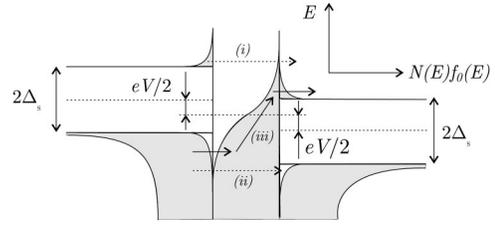
FIG. 7. Semiconductor-diagram representation of tunnel and scattering rates in a double-barrier junction at bias voltage  $eV = \Delta_S$ . The energy conserving processes (i) and (ii) are, in the case of inelastic scattering, complemented by process (iii).
