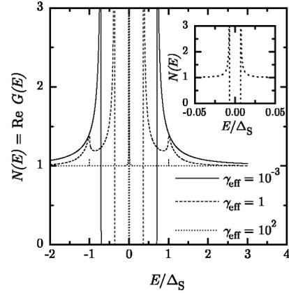
FIG. 2. Normalized density of states in the interlayer at  $T=0$  for several values of the suppression parameter  $\gamma_{\text{eff}}$ . The inset shows the minigap that is present for  $\gamma_{\text{eff}} = 10^2$  on a smaller scale.
