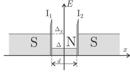
FIG. 1. Schematic representation of the double-barrier SINIS structure. Two superconducting electrodes (S) are separated by two delta-shaped potential barriers ( $I_1$  and  $I_2$ ) and a normal metal interlayer (N). The position dependence of the pair potential has been indicated by shading.
