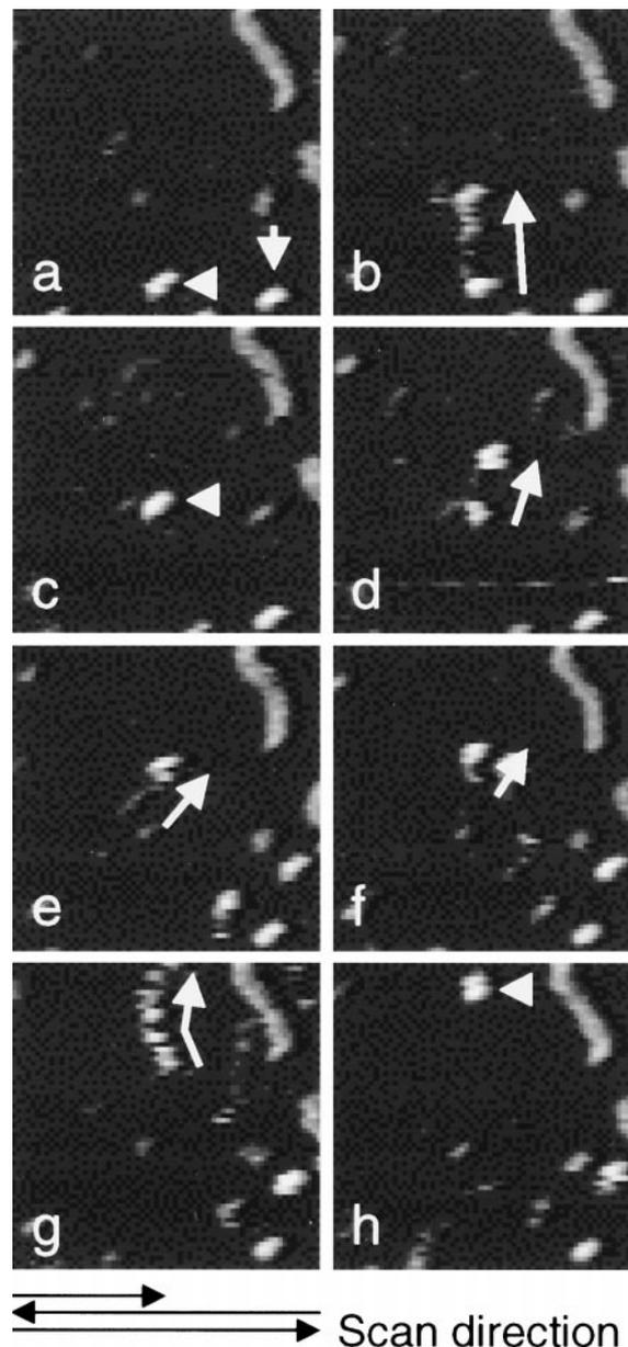
FIGURE 4 Sequence of eight successive topography images obtained by tapping-mode AFM at times  $t = 1, 2, 3, 4, 5, 6, 11,$  and  $12 \text{ min}$ . Two photolyase molecules are indicated by white arrows in *a*. White arrows in *b–h* indicate the movement of one photolyase molecule. The black arrows indicate the scan direction of the tip. Scan area,  $250 \times 250 \text{ nm}^2$ ;  $z$  range, 4 nm.
