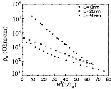
Fig.1. Temperature dependencies of  $c$ -axis PBCO resistivity in YBCO/PBCO/Au contacts resistances for several barrier thicknesses  $L$ .
