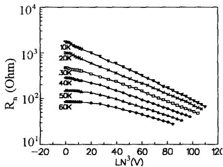
Fig.2.  $R(V)$  dependencies of YBCO/PBCO/Au structures with 20 nm thick PBCO barrier.
