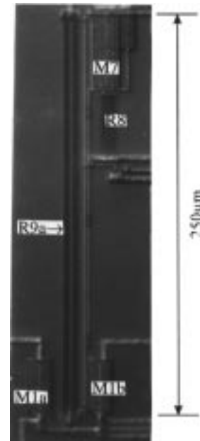
Fig. 7. A transconductor using a merged device with maximized tune range, suitable for AGC applications.
