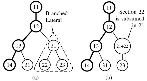
Fig. 2. Example of the difficulties encountered when the ST model is applied. (a) After choosing the main line (shown in bold.), the lateral rooted at node 21 has two branches. (b) Section 22 is subsumed in node 21.
