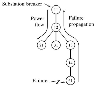
Fig. 1. Simple seven-section feeder [2].
