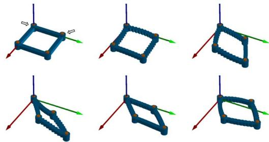
Fig. 10. Simulation results for the 2-DoF flexible closed kinematic chain.
