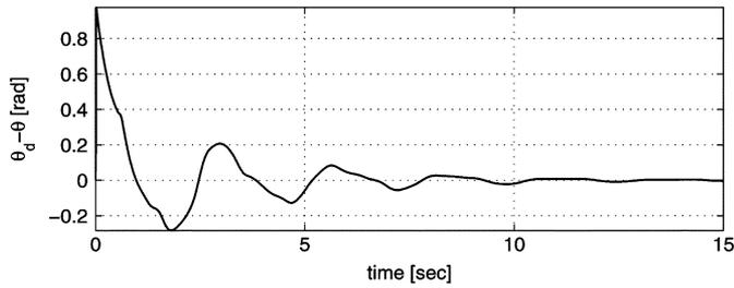
Fig. 4. Evolution in time of joint rotation error  $\theta_d - \theta$ , in radians.
