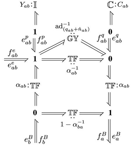
Fig. 3. Bond graph of the finite-dimensional approximation of the flexible link on  $\mathcal{Z}_{ab} \subset \mathcal{Z}$ .
