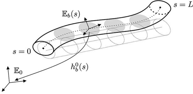
Fig. 1. Schematic representation of a flexible link in the deformed and unstressed configurations.
