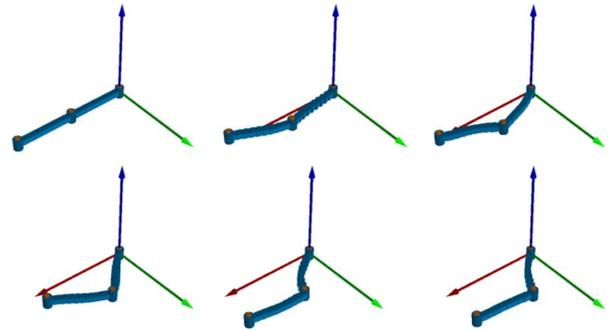
Fig. 9. Simulation results for the 2-DoF manipulator with flexible links.
