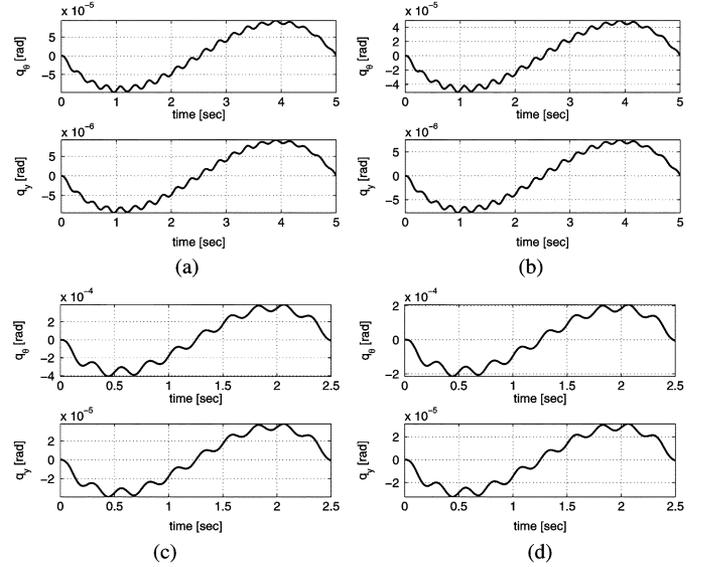
Fig. 7. PP-s and PP-f maneuvers. (a) PP-s,  $s = L/4$ . (b) PP-s,  $s = L/2$ . (c) PP-f,  $s = L/4$ . (d) PP-f,  $s = L/2$ .
