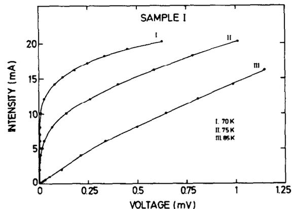
Fig. 3. AC current amplitude versus voltage of  $\text{YBa}_2\text{Cu}_3\text{O}_{7-\delta}$  (sample I) for  $\nu = 3$  Hz and temperatures above and below
