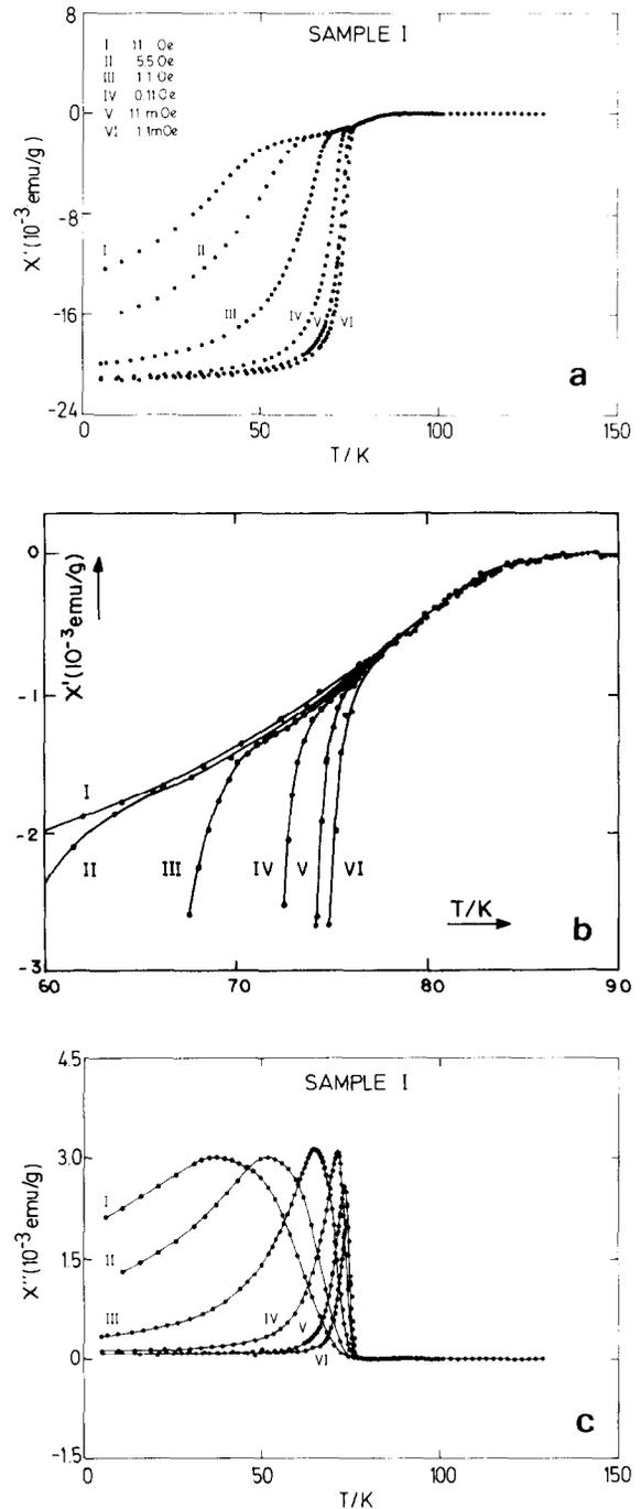
Fig. 1. In-phase (a) and out-phase (c) ac magnetic susceptibility of  $YBa_2Cu_3O_{7-\delta}$ , sample I, for  $\nu = 121$  Hz. The curves labeled I to VI correspond to different exciting amplitudes. In (b) the region close to the superconducting percolative transi-
