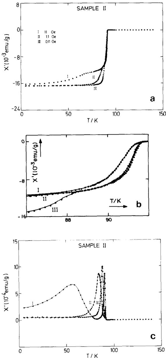
Fig. 2. In-phase (a) and out-phase (c) ac magnetic susceptibility of  $\text{YBa}_2\text{Cu}_3\text{O}_{7-\delta}$ , sample II, for  $\nu = 121$  Hz. The curves correspond to different exciting amplitudes. In (b) the region
