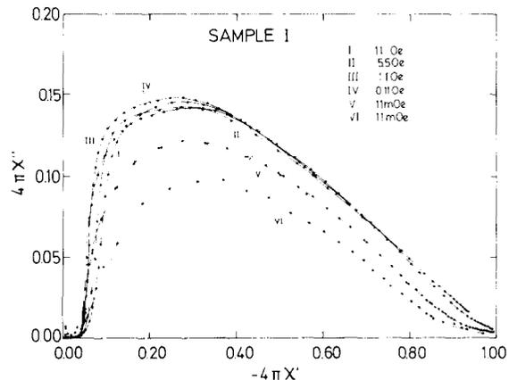
Fig. 4.  $\chi''$  versus  $\chi'$  magnetic susceptibility of  $YBa_2Cu_3O_{7-\delta}$  (sample I;  $\nu = 121$  Hz) for temperatures below  $T_c = 75$  K. Both axes have been normalized so that for the lowest exciting
